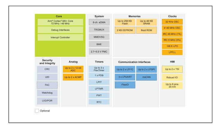
View additional information for 72MHz, 5V Main Stream CM0+ MCU with NXP Touch (TSI) and CAN Control.
