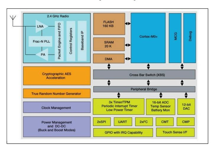
View additional information for Kinetis® KW20Z-2.4 GHz 802.15.4 Wireless Radio Microcontroller based on Arm® Cortex®-M0+.
