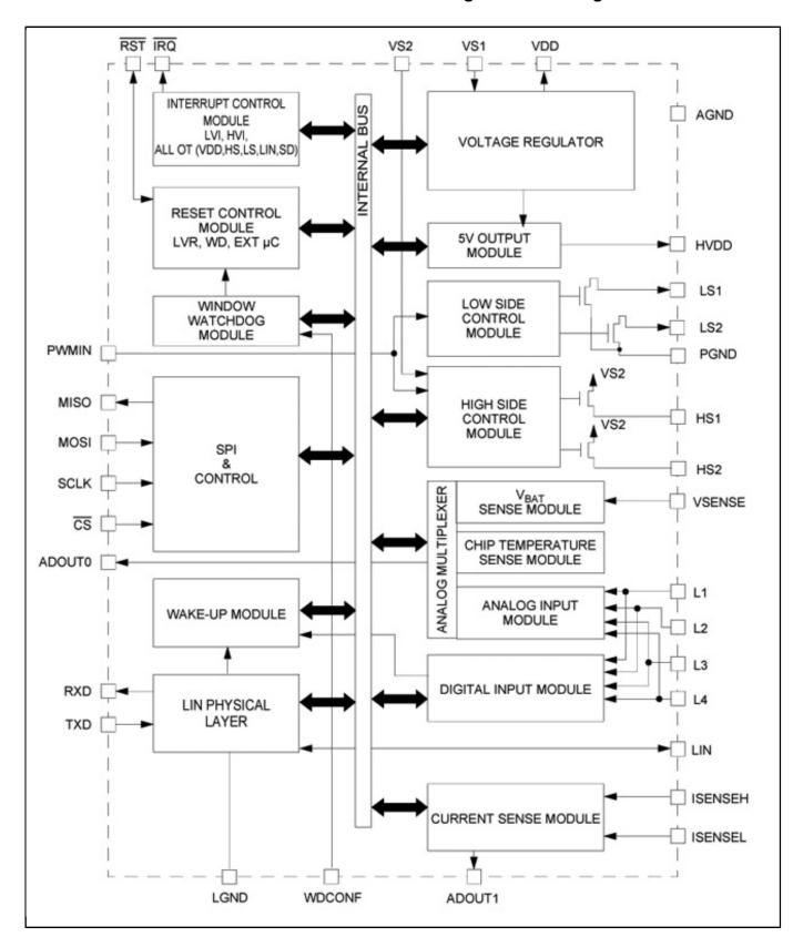
Freescale MC33912 Network Transceivers Block Diagram Block Diagram
