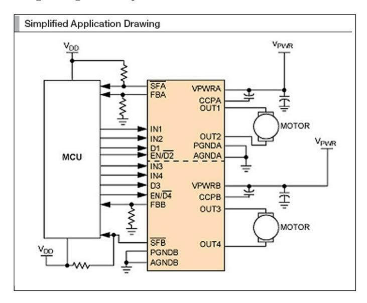
View additional information for MC34932/S H-Bridge, Brushed DC Motor Driver, 5-36 V, 5 A, 11 kHz/20 kHz.
