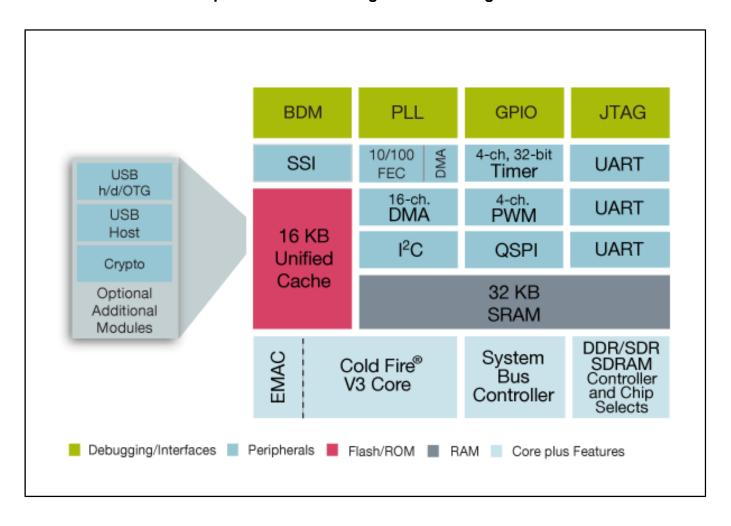
View additional information for Coldfire V3 Microprocessor with Ethernet, USB and Encryption.
