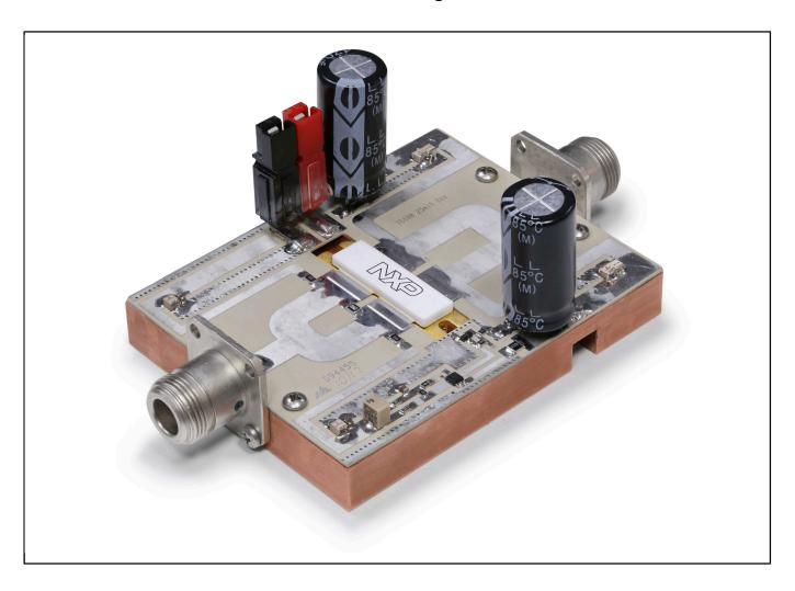
View additional information for 750 W CW over 700-1300 MHz, 50 V RF Power LDMOS Transistor.
