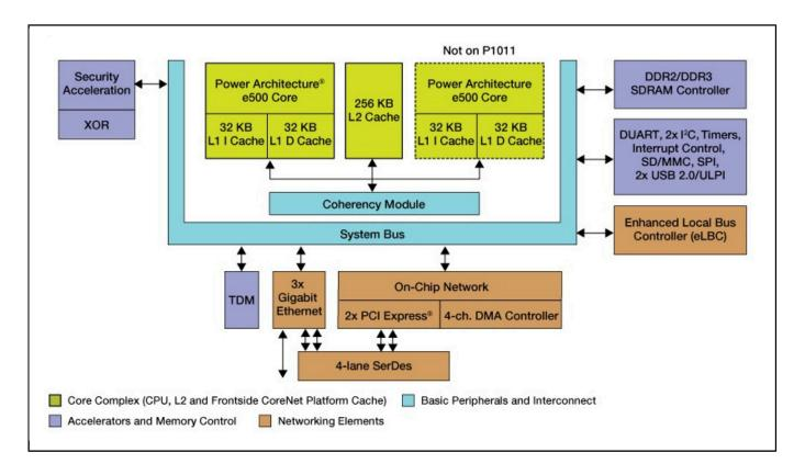
View additional information for QorlQ® P1020 and P1011 Dual- and Single-Core Communications Processors.
