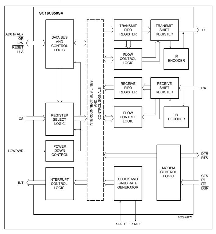
View additional information for 1.8 V Single UART, 20 Mbit/s (max.) with 128-Byte FIFOs, Infrared (IrDA), and XScale VLIO Bus Interface.
