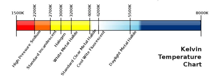
Color temperature is a quanitiave measure of how white a light source is compared to others. The higher numbers are associated with the "cooler", "bluer" shades of white, lower numbers are associated with the "warmer" or "soft white" shades of white.
