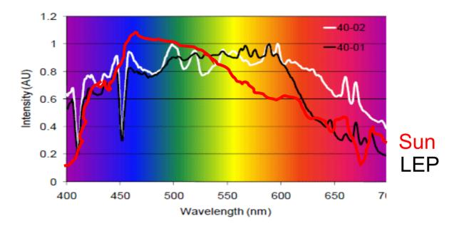
Spectral power distribution is a quantitative measure of how closely the frequency spectrum of the light source compares to that produced by the sun. Spectral distribution helps with color rendering and is required by plant life in aquariums and artificial growing environments.
