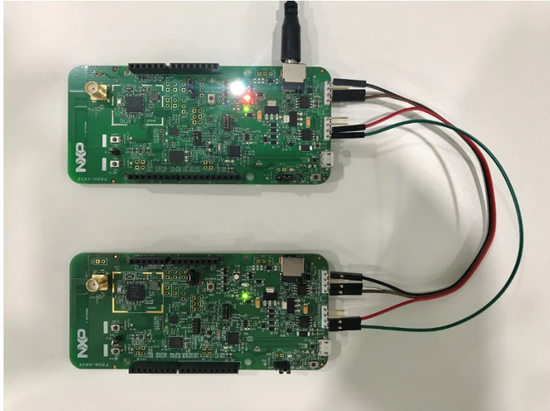
Figure 1. Using FRDM-KW36 DK boards to debug LIN/CAN communication
