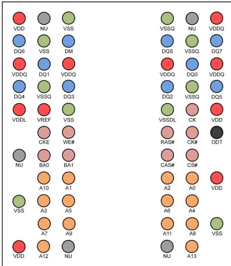
Figure 2. Example DDR2 Memory Configuration x8 (View Through Package)
