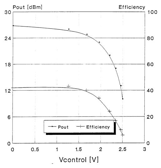
Vs=3.6V, F=1.88GHz, Pin=3dBm "R06\_V05\V007"
