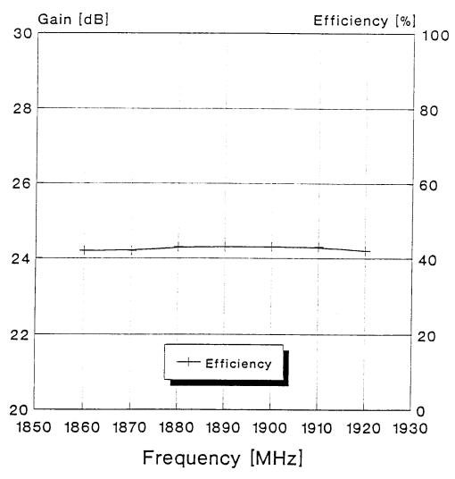
Vs=3.6V, Pin=3dBm, Pout=26dBm "R06\_V04\V005"
