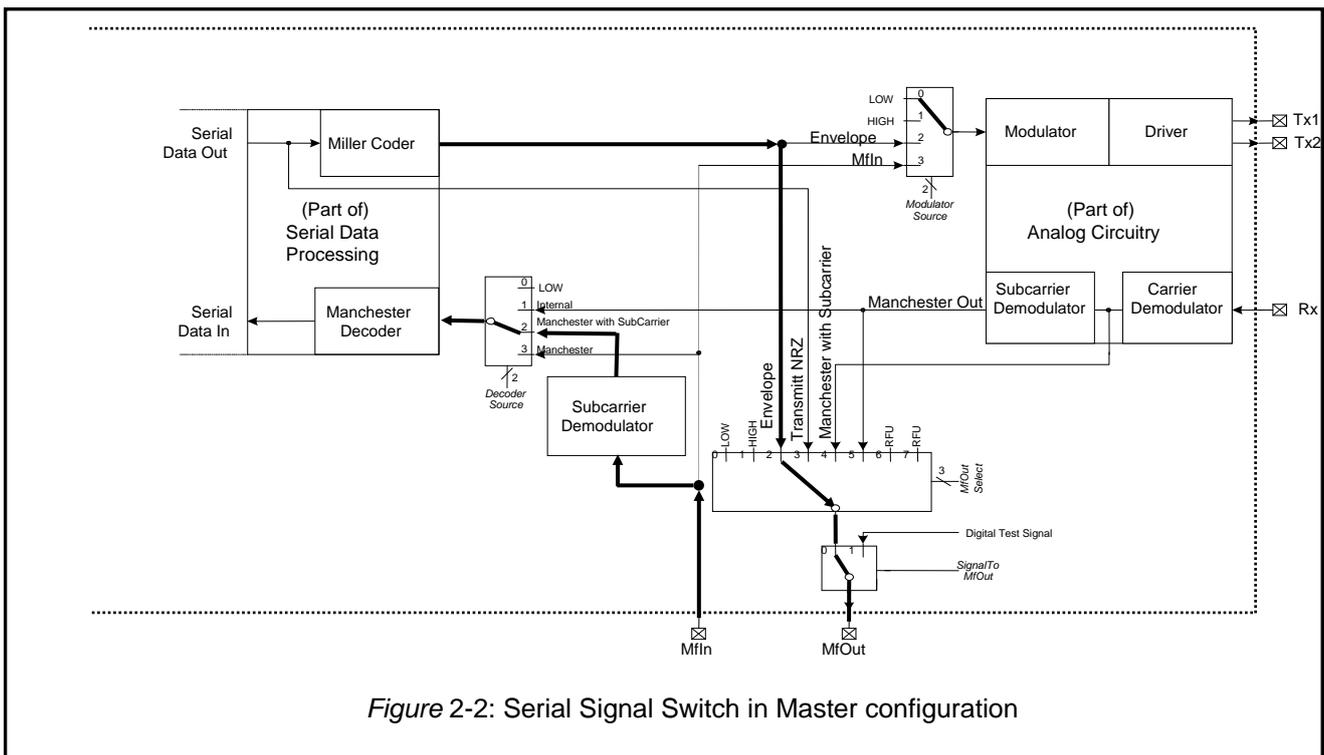
Figure 2-2: Serial Signal Switch in Master configuration
