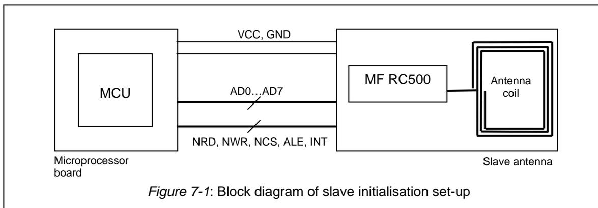
Figure 7-1: Block diagram of slave initialisation set-up
