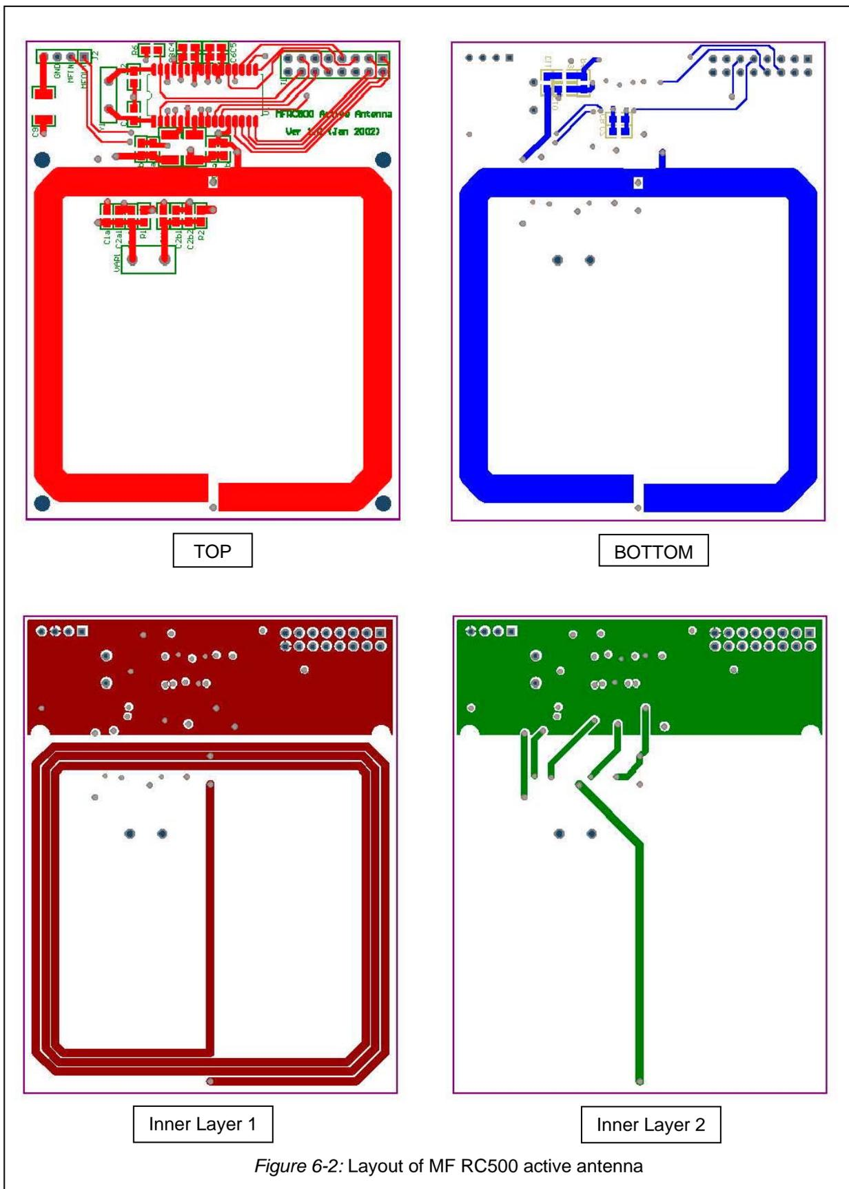
Figure 6-2: Layout of MF RC500 active antenna
