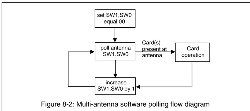
Figure 8-2: Multi-antenna software polling flow diagram
