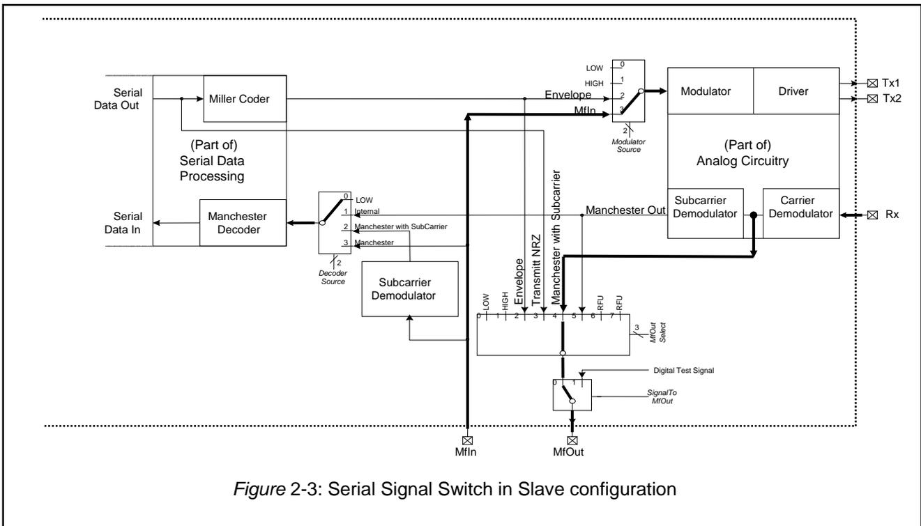
Figure 2-3: Serial Signal Switch in Slave configuration
