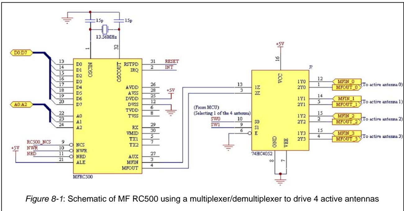
Figure 8-1: Schematic of MF RC500 using a multiplexer/demultiplexer to drive 4 active antennas
