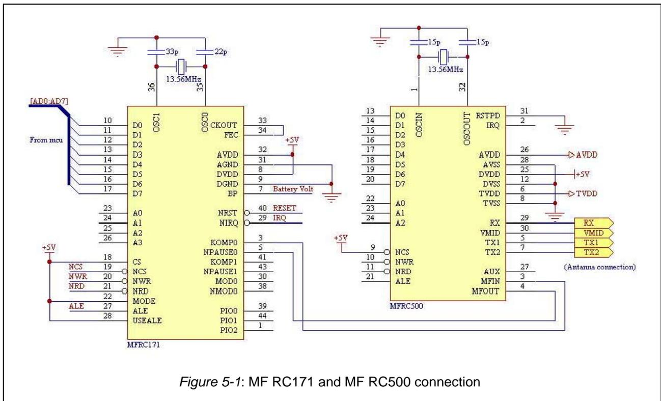
Figure 5-1: MF RC171 and MF RC500 connection
