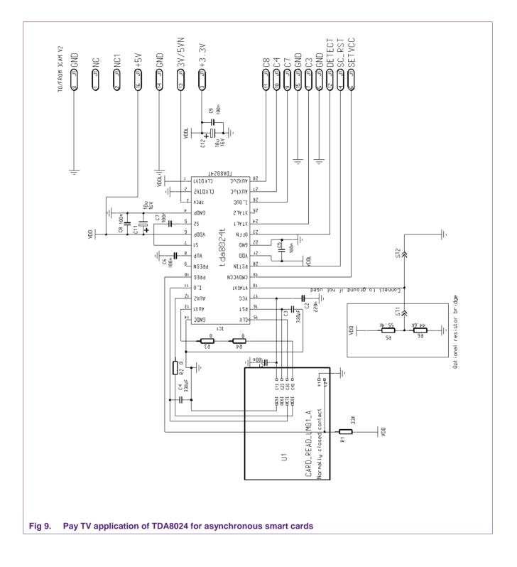
In this case the clock signal is coming from the NDS device and so the CLK frequency has been programmed as XTAL/1.
