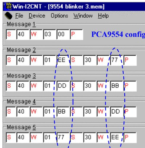
PCA9554 configuration register (I/O configured as outputs)
