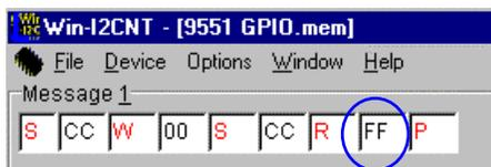
Input register value is 1111111<sub>b</sub> or FF<sub>H</sub>. All the pins are read with a Logic Level 1
