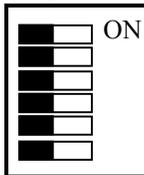
All the switches are OFF, MUX\_IN[F:A] = 000000<sub>b</sub> or 00<sub>H</sub>
