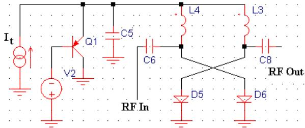
**Figure 5 . Circuit with Two Diodes and Hybrid.**
