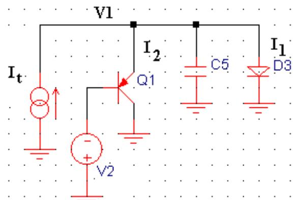
Figure 4. Transistor Shunt.  $V2 < 200$  mV.
