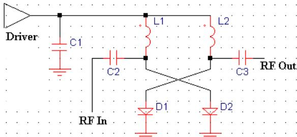
**Figure 1. Commonly Used Attenuator. Diodes are BAP50-05.**
