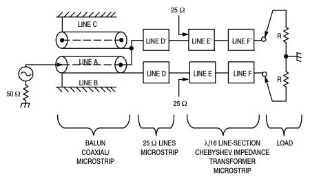
FOR LINE A:  $Z_0=50~\Omega$ ;  $L=1799~\text{MILS};~\epsilon_f=2.10$  LINES B AND C:  $Z_0=30~\Omega$ ;  $L=1799~\text{MILS};~\epsilon_{eff}=2.23$  LINES D AND D':  $Z_0=25~\Omega$ ;  $L=750~\text{MILS};~\epsilon_{eff}=2.23$  LINES E AND E':  $Z_0=61.5~\Omega$ ;  $L=464~\text{MILS};~\epsilon_{eff}=2.10$  LINES F AND F':  $Z_0=20.3~\Omega$ ;  $L=441~\text{MILS};~\epsilon_{eff}=2.31$
