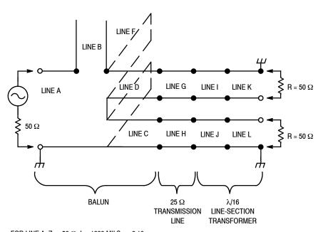
FOR LINE A:  $Z_0=50~\Omega$ ; L = 1888 MILS;  $\epsilon_{ff}$  2.10 LINE B:  $Z_0=25~\Omega$ ; L = 1810 MILS;  $\epsilon_{ff}$  2.23 LINES E AND F:  $Z_0=30~\Omega$ ; L = 1772 MILS;  $z_0=2.30~\Omega$ ; L = 1546 MILS;  $z_0=2.30~\Omega$ ; L = 1546 MILS;  $z_0=2.30~\Omega$ ; L = 140 MILS;  $z_0=2.30~\Omega$ ; L = 140 MILS;  $z_0=2.30~\Omega$ ; L = 466 MILS;  $z_0=2.30~\Omega$ ; L = 443 MILS;  $z_0=2.30~\Omega$
