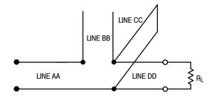
FOR LINE AA:  $Z_A$  = 50  $\Omega$ ;  $L_A$  = 1888 MIL;  $\epsilon_{ff}$  = 2.10 LINE BB:  $Z_B$  = 25  $\Omega$ ;  $L_B$  = 1810 MIL;  $\epsilon_{eff}$  = 2.23 LINE CC: 2 $Z_E$  = 35.8  $\Omega$ ;  $L_E$  = 1772 MIL;  $\epsilon_{ff}$  = 2.33 LINE DD: 2 $Z_D$  = 50  $\Omega$ ;  $L_D$  = 1546 MIL;  $\epsilon_{eff}$  = 2.23
