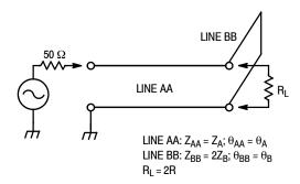
SYMMETRIC BALUN INPUT EQUIVALENT CIRCUIT
