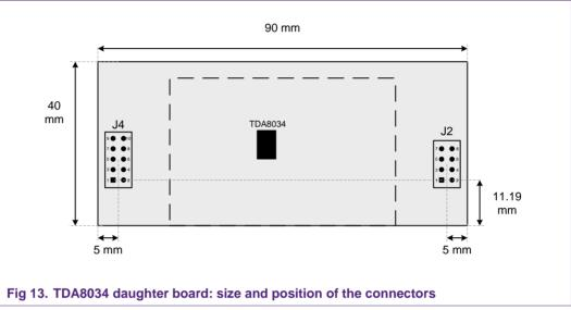
All the contact interfaces needed to drive the TDA8034 are available on the J2 and J4 connectors. These signals are defined below.
