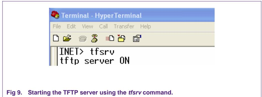
Fig 9. Starting the TFTP server using the *tfsrv* command.
