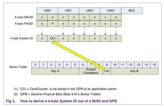
This system ID must be created when the card is issued or personalized as shown in <u>Fig</u> <u>4</u>. The GPB should be stored in a Sector Trailer that is not going to be changed later on. It could be the Sector Trailer of the first sector being used by the application.
