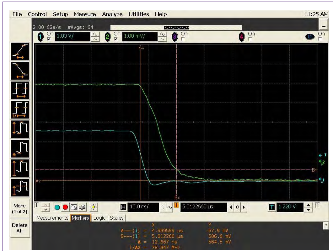
3.0Vrms, 100KHz and 50% duty cycle pulse applied on VCC pin, measured from 50% of input pulse to 10% of max. output power
