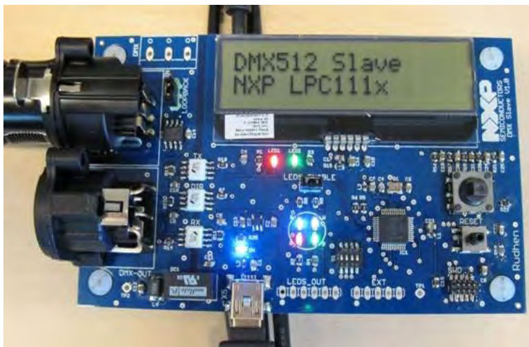
Fig 3. NXP DMX512 slave demo board
