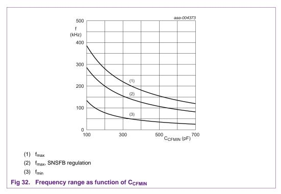
The oscillator frequency depends on the charge and discharge current of the capacitor on the CFMIN pin. The charge and discharge current consists of a fixed part which determines the minimum frequency and the SNSFB and SSHBC/EN pins control functions drive a variable part.
