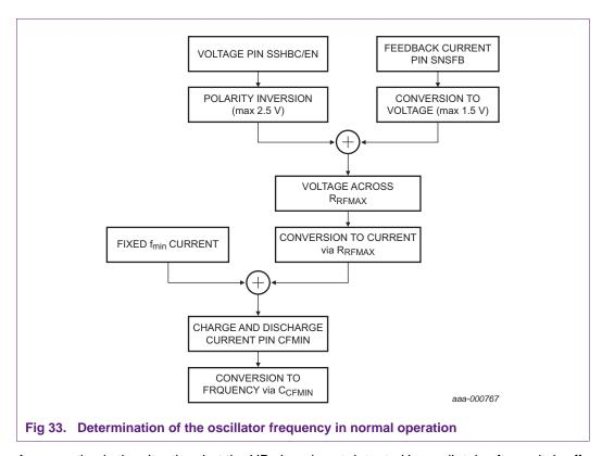
An exception is the situation that the HB slope is not detected immediately after switch-off. Until the HB slope is detected, only a small current source of 30  $\mu$ A charges the oscillator capacitor.
