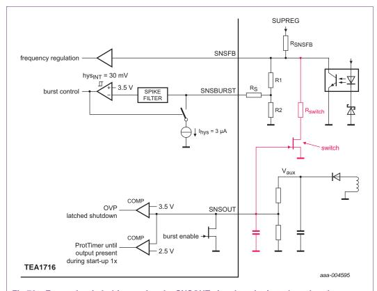
Fig 76. External switch driven using the SNSOUT signal to obtain a short duration
