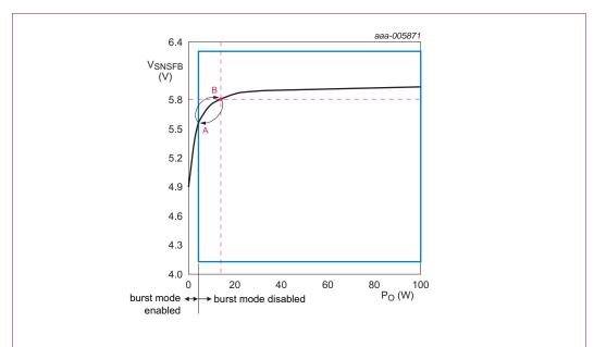
Fig 80. Using an external burst mode enable/disable function that is set at a lower power level than the preset SNSBURST level
