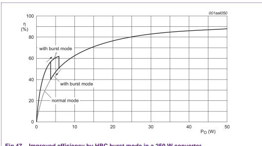
Fig 47. Improved efficiency by HBC burst mode in a 250 W converter
