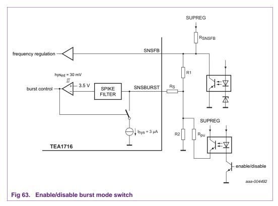
The enable/disable function can also be used to implement a better defined transition for entering and leaving burst mode operation. See Section 11.11.
