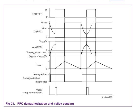
The valleys are detected at the SNSAUXPFC pin. An auxiliary winding on the PFC coil provides a measurement signal on the SNSAUXPFC pin. It gives a reduced and inverted copy of the MOSFET drain voltage. When a valley of the drain voltage (top SNSAUXPFC voltage) is detected, the MOSFET is switched on.
