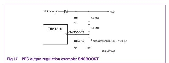
The boost output voltage value is set between the PFC output voltage and the SNSBOOST pin using a resistor divider. When in regulation, the SNSBOOST voltage is kept at 2.5 V.
