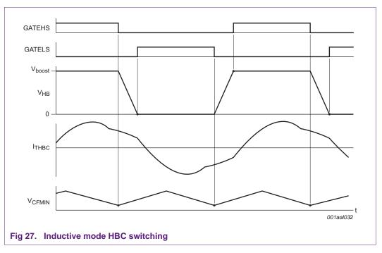
The time required for the transition of the HB depends on the amplitude of the resonant current at the moment of switching. There is a (complex) relationship between the amplitude, the frequency, the boost voltage and the output voltage. Ideally, the IC switches on the MOSFET when the transition of the HB has reached its end value. It must not wait longer, especially at high output load to prevent a swing back of the HB voltage.
