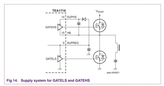
Both HBC drivers have a strong current source capability and an extra strong current sink capability. In general HBC operation, fast switch-on of the external MOSFET is not critical, as the HB node swings automatically to the correct state after switch-off. Fast switch-off, however, is important to limit switching losses and prevent delay especially at high frequency.
