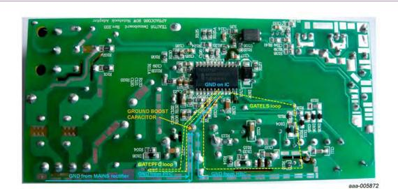
Fig 90. Grounding layout example with star point at the boost capacitor
