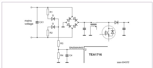
Fig 26. Example of a peak sensing SNSMAINS measurement circuit (adding two diodes D)
