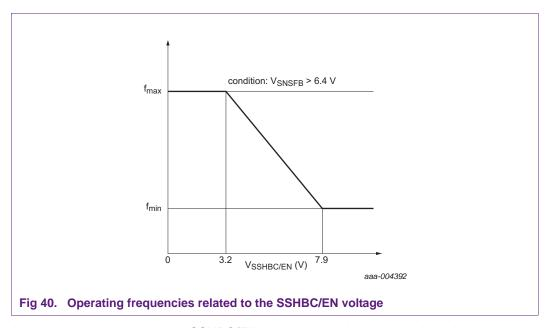
At start-up, the voltage on the SSHBC/EN pin is low which corresponds to the maximum frequency. During the soft-start procedure, the external capacitor is charged. The voltage on the SSHBC/EN pin rises and the frequency decreases. The contribution of the soft-start function ends when the SSHBC/EN pin exceeds 7.9 V.
