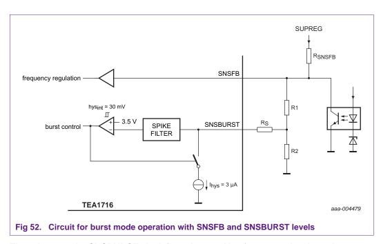
The voltage on the SNSBURST pin defines the transition from operational supply state (burst-on period) to burst stop state (burst-off period) and back.
