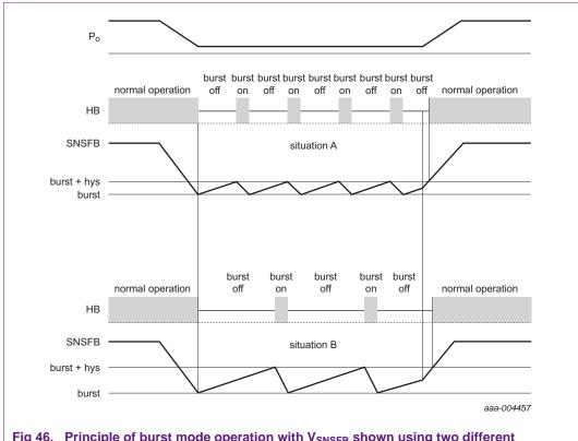
Fig 46. Principle of burst mode operation with V<sub>SNSFB</sub> shown using two different hystereses
