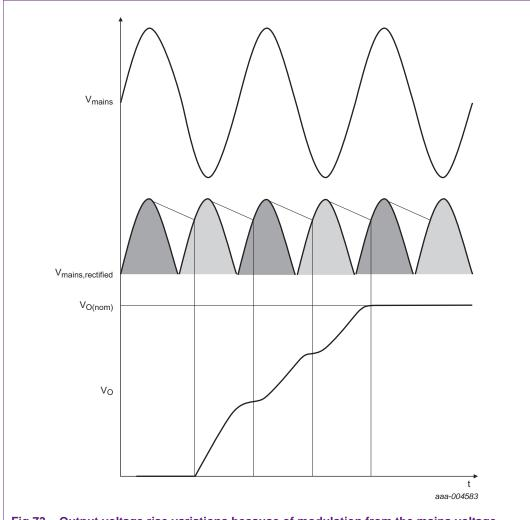
Fig 73. Output voltage rise variations because of modulation from the mains voltage
