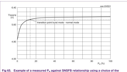
Fig 65. Example of a measured P<sub>o</sub> against SNSFB relationship using a choice of the transition point
