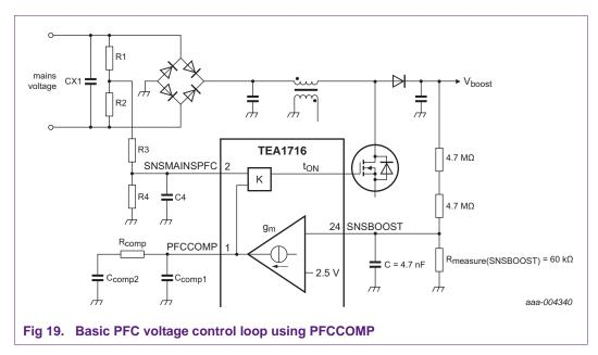
The transfer function has a pole at 0 Hz, a zero at  $R_{comp}/C_{comp2}$  and a pole again at  $C_{comp1}/C_{comp2}$ . Set the zero frequency to 10 Hz while the next pole frequency is at 40 Hz. The zero point and pole frequencies of the compensation network can be calculated using Equation 11 and Equation 12.
