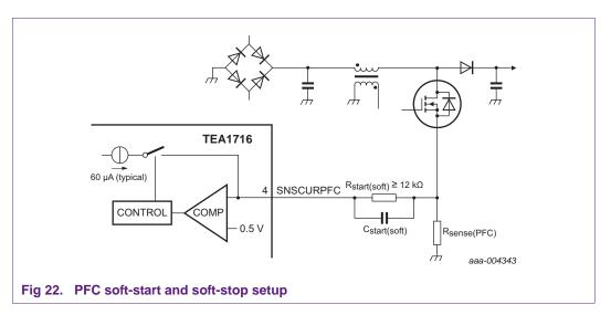
A resistor and a capacitor between the SNSCURPFC pin and the current sense resistor  $R_{\text{sense(PFC)}}$  set both functions.
