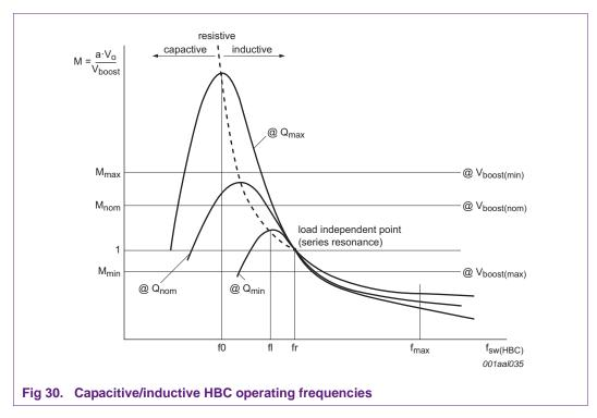
The typical slowing of the oscillator combined with the discharging of the SSHBC/EN pin indicates the CMR of the TEA1716.
