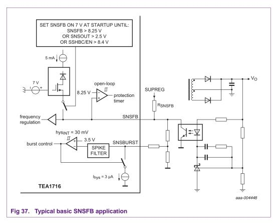
The frequency regulation function senses the voltage on SNSFB.
