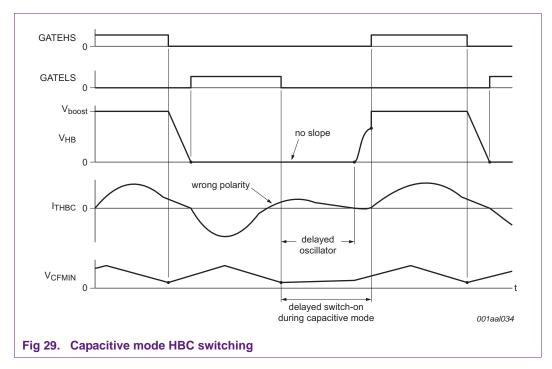
The adaptive non-overlap system of the TEA1716 always waits until the slope at the half-bridge node starts. It guarantees safe/best switching of the MOSFETs in all circumstances. In capacitive mode, it can take half the resonance period before the resonant current changes back to the correct polarity and starts charging the half-bridge node. The oscillator remains in slow charging current mode until the half-bridge slope allows this relatively long waiting time (see Section 9.4.2 and Figure 34).
