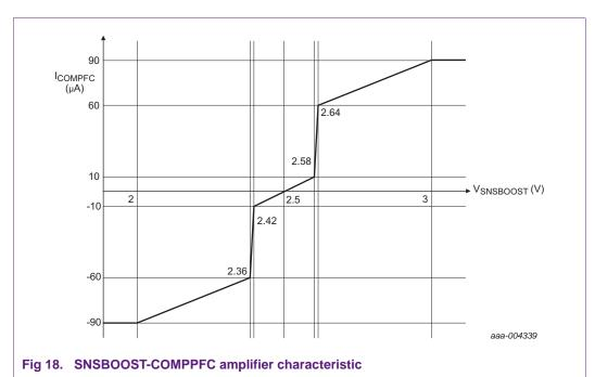
The transconductance amplifier output is available at the COMPPFC pin for adding an external loop compensation network. The current from the error amplifier results in a loop voltage on the COMPPFC pin. This COMPPFC voltage and the voltage on the SNSMAINS pin, determine the PFC switch-on time.
