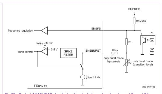
Fig 55. Typical SNSBURST circuit showing the independent functions of Rs and R2
