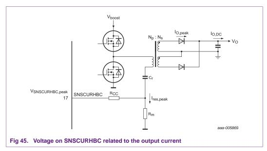
The relationship between the voltage on the SNSCURHBC pin and the primary converter current is defined by measuring resistor  $R_{\rm m}$ .
