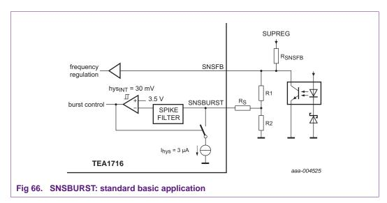
The SNSBURST comparator level is 3.5 V.
