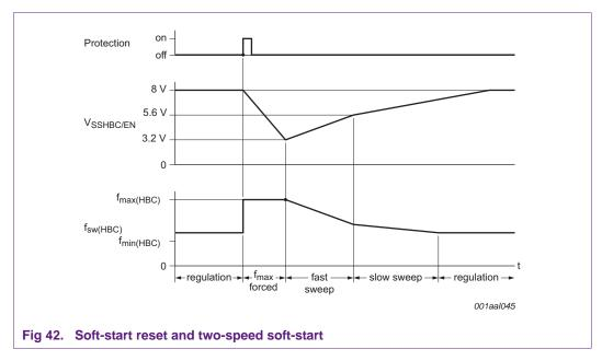
The soft-start reset is also used to ensure a safe start-up at maximum frequency when SSHBC/EN or a restart enable the HBC. The soft-start reset is not used when the operation has been stopped for burst mode.
