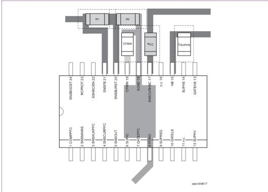
Fig 91. PCB layout: connecting the SGND, PGND, CFMIN, SNSCURHBC and SNSBURST pins
