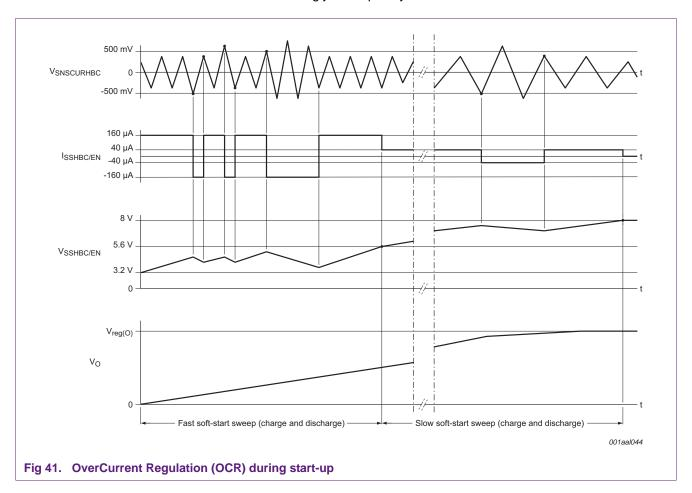
The slow charge or discharge speed is used for the lower frequency range where V<sub>SSHBC/EN</sub> is above 5.6 V. In the lower frequency range, the current in the converter reacts strongly to frequency variations.
