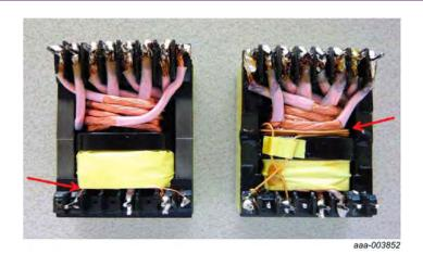
Fig 7. Transformer auxiliary winding on primary side (left, not preferred) and secondary side (right)
