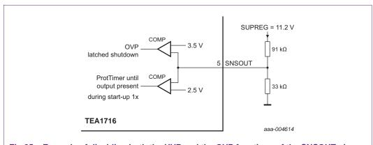
Fig 85. Example of disabling both the UVP and the OVP functions of the SNSOUT pin
