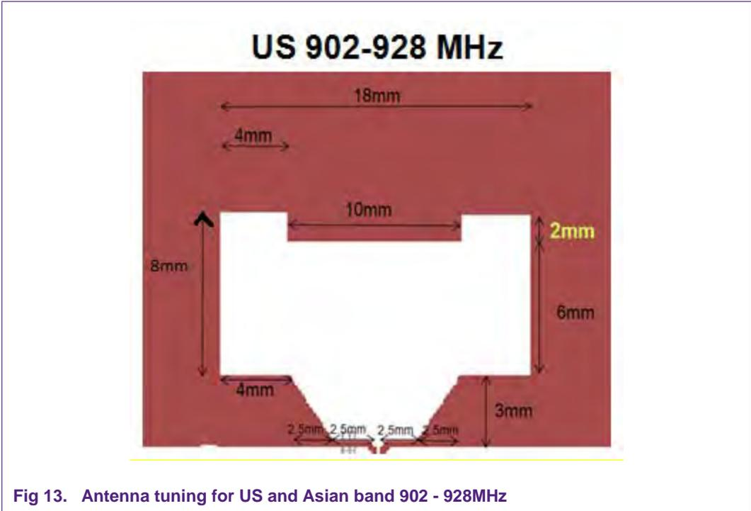
Fig 13. Antenna tuning for US and Asian band 902 - 928MHz
