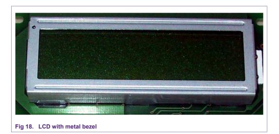
The metal bezel, which is used in LCD applications with the driver somewhere on the board, provides also shielding for EMI and ESD, provided that it is connected to GND.
