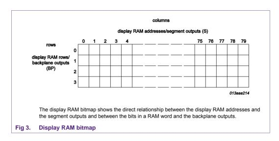
A logic 1 in the RAM bitmap indicates the on-state of the corresponding LCD element; similarly, a logic 0 indicates the off-state.
