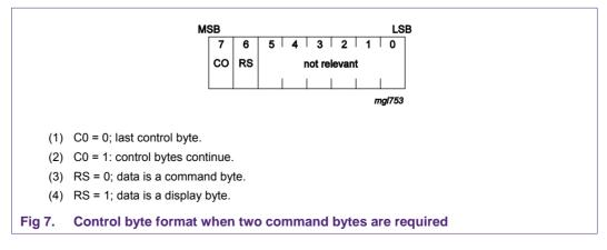
This command structure is used for the xxx34 and xxx33 types. The possible addresses here range from 0 to 79.
