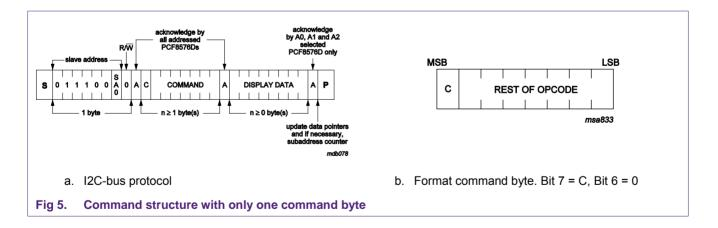
With 6 bits up to  $2^6 = 64$  addresses can be used. In 1:4 multiplex mode, this allows for 256 segments. This control structure is used for the xxx62 and xxx76 types, where the addresses range from 0 to 39.
