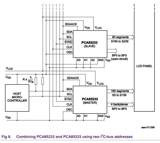
Due to the differences in command structure, it is not possible to combine LCD drivers with command structure version 1, with drivers using version 2 or 3.
