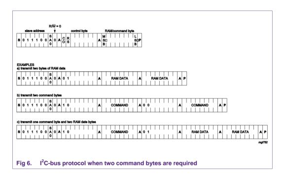
After acknowledgement, the control byte is sent defining whether the next byte is a command or contains RAM information. The control byte contains also an RS bit (register select) at position b6. The other bits are don't care. This is shown in <u>Fig 7</u>. In between two command bytes always this control byte is included. Once RAM data is started to be sent, no further control bytes are required.
