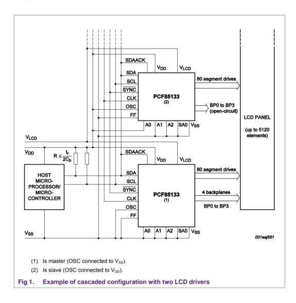
The lower device in Fig 1 is the master. By connecting pin OSC to  $V_{SS}$ , the internal oscillator is enabled. On pin CLK the clock signal (from the internal oscillator) is available to be used as input for slave devices in the cascade. Of course it is also possible to use an external signal, in that case pin OSC of the master must be connected to  $V_{DD}$ .
