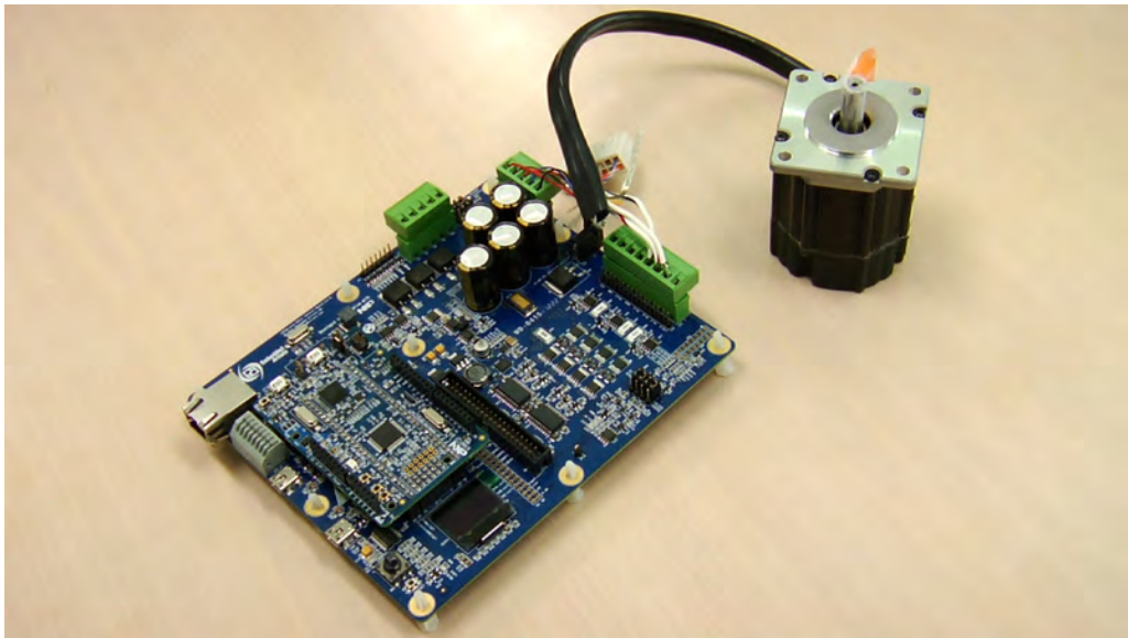
Fig 22. PMSM motor control demo setup
