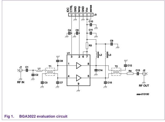
The power supply is applied on the Vcc pin of connector J3 and is applied to the BGA3022 via chokes L2 and L3 which provides RF blocking to the supply line. Capacitors C9, C10 and C11 are supply decoupling capacitors, where C4 and C5 are decoupling capacitors for the control lines.
