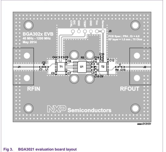
For optimum distortion performance it is important to have enough ground vias underneath and around the MMICs ground pins. This lowers the inductance to the ground plane. The evaluation board is made with two layer FR4 material.
