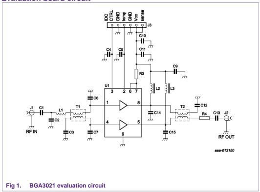
The power supply is applied on the Vcc pin of connector J3 and is applied to the BGA3021 via chokes L2 and L3 which provides RF blocking to the supply line. Capacitors C9, C10 and C11 are supply decoupling capacitors, where C4 and C5 are decoupling capacitors for the control lines.
