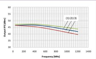
b.  $f2 = f1 \pm 6$  MHz, output power = 10 dBm per frequency.
