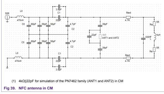
The simulation and measurement result is shown in Fig 40. The resonance frequency in CM is approximately 16MHz.
