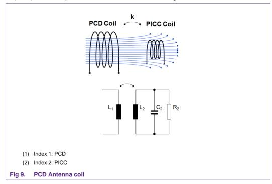
The index 2 indicates the parameters of the PICC. Here the PICC is taken as given, i.e. the parameters with the index 2 cannot be modified. This is another simplification, but also refers to the reality, where the reader antenna optimization does not allow to change card parameters.
