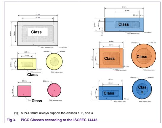
The PCD antenna coil sizes are not specified. So for ISO/IEC 14443 compliant readers all different sizes of antenna coils from a few 10 mm<sup>2</sup> up to 20cm diameter can be found in various shapes.
