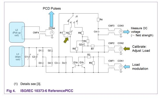
Some ReferencePICCs, which are commercially available (e.g. Fig 5), are pre-calibrated and equipped with several jumper options to address the most relevant tests with a single ReferencePICC.
