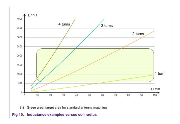
On the other hand, the number of turns defines the relationship of voltage level versus current level. Especially for the load modulation (see Fig 11) it might be helpful to increase the number of turns on the PCD antenna coil.
