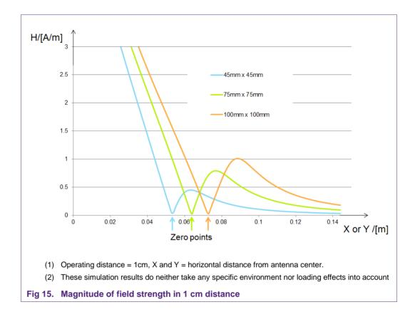
**Note:** The field strength is not the same for all three antennas, but has been adjusted individually to achieve the maximum allowed field strength for each antenna.
