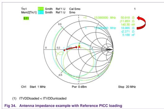
PICC is place closely to the antenna to achieve the maximum possible coupling between PCD and PICC.
