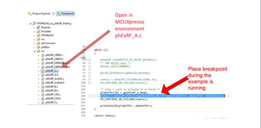
Fig 56. Placing breakpoint to pause example to change register
