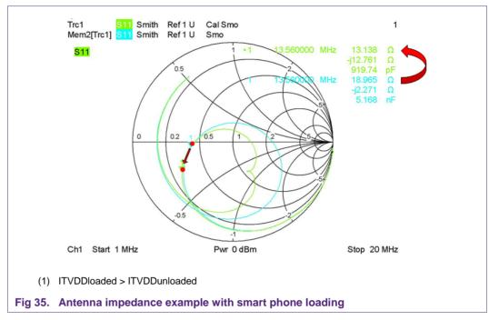
As can be see, in this case of metal loading the ITVDD must increase, since the overall impedance gets lower:
