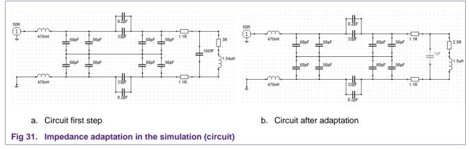
With these adapted values of the antenna coil the last step of the final tuning can be done:
