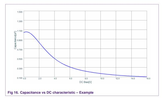
This capacitor has a nominal value of  $1\mu$ F at 0V, but falls to 300nF at 6V, which is the operating voltage on VUP. Then the behavior of the DC/DC is not the expected one.
