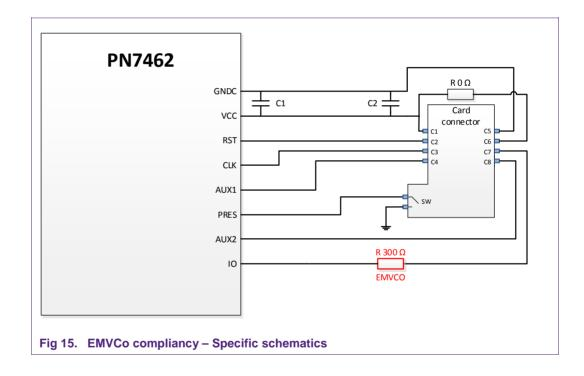
The reason to add this Resistor is to be compliant with the IO current limitation specification:
