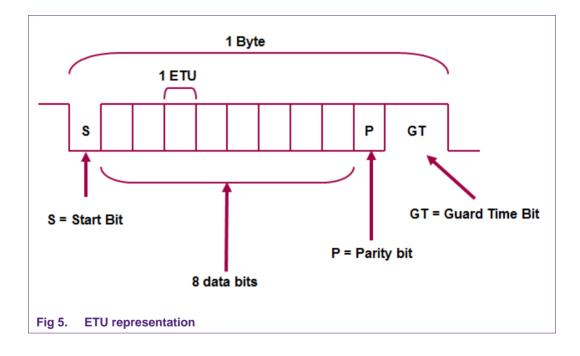
The default length for one ETU is set by ISO7816 to 372 Clock cycles (referenced to the clock sent to the smart card). This is the value to be used during card activation (ATR reception).
