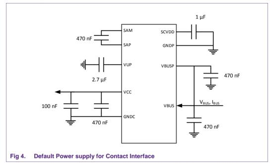
The DC/DC converter operates as a charge pump using capacitors on SAx pins, and Vup. With these pins the converter can operate as a voltage follower or doubler. This allows to use a VDDP down to 3 V to generate 5V, or down to 2.7V to generate 3V, and then allows to use the same voltage level for VBUS and VBUS\_P.
