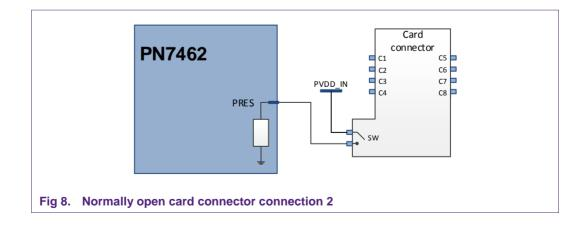
This is the recommended configuration for normally open card connector presence switch.
