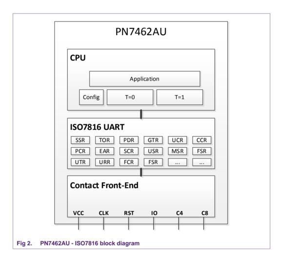
The ISO7816 UART block is a set of registers and digital management. It fully handles ISO7816 low level as specified in ISO7816-3.
