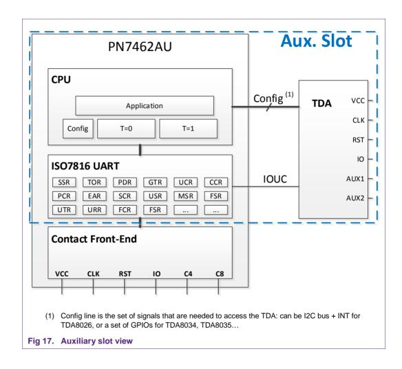
In ISO7816 UART block within the PN7462AU, the auxiliary slot is generally called slot 2, while the main slot is called slot 1.
