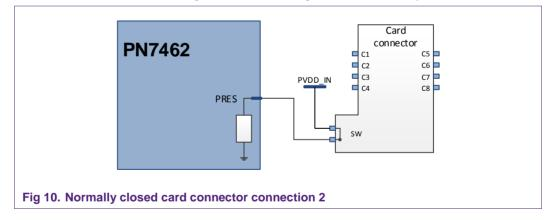
This is the recommended configuration for normally closed card connector presence switch.
