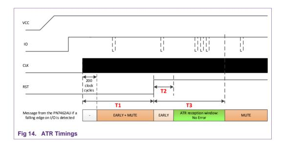
T1, T2 and T3 timers are configurable through Contact Registers: T1 is set by the registers CT\_MCLR\_LSB\_REG and CT\_MCLR\_MSB\_REG T2 is 200 clock cycles plus the value configured through CT\_ECR\_REG T3 is set through CT\_MCHR\_LSB\_REG and CT\_MCHR\_MSB\_REG Each value is set in number of clock cycles.
