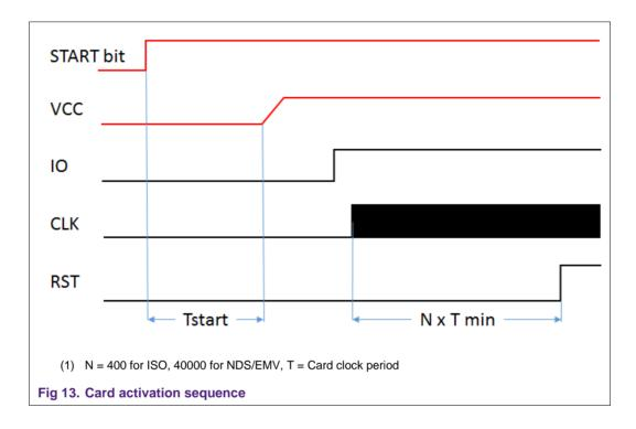
The delay Tstart is a PN7462 internal delay: this time is used by the DC/DC to start, and is approximately 20 ms.
