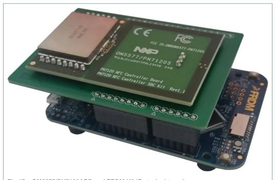
Fig 17. OM5577/PN7120ARD and FRDM-K64F stacked together
