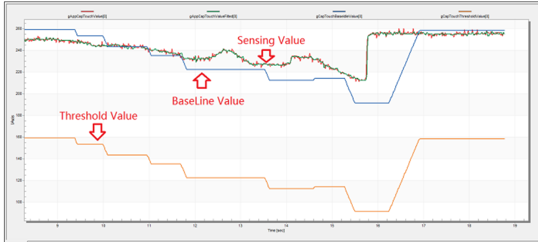
Fig 10. Self-adapted baseline and asymmetric debounce filter diagram
