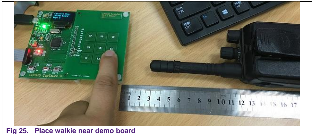
Fig 25. Place walkie near demo board
