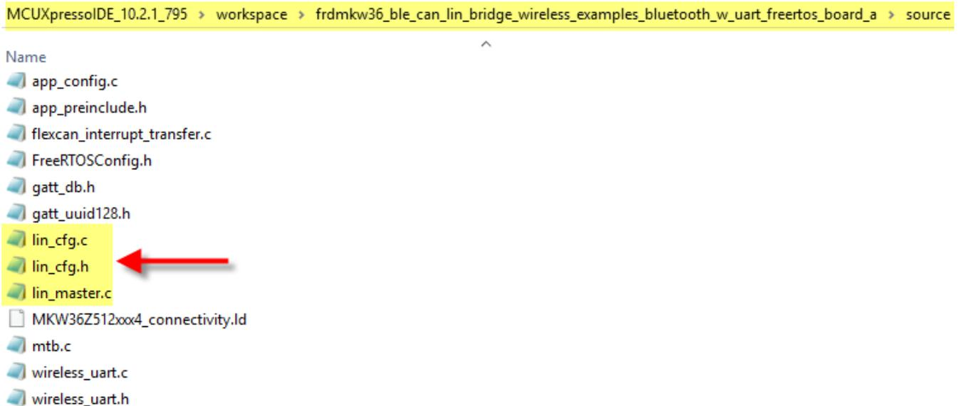
**Figure 19.** LIN master application files added in MCUXpresso workspace
