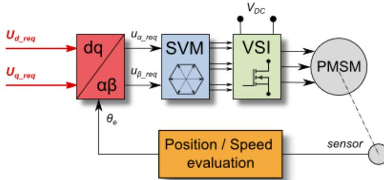
Figure 27. Voltage FOC control mode
