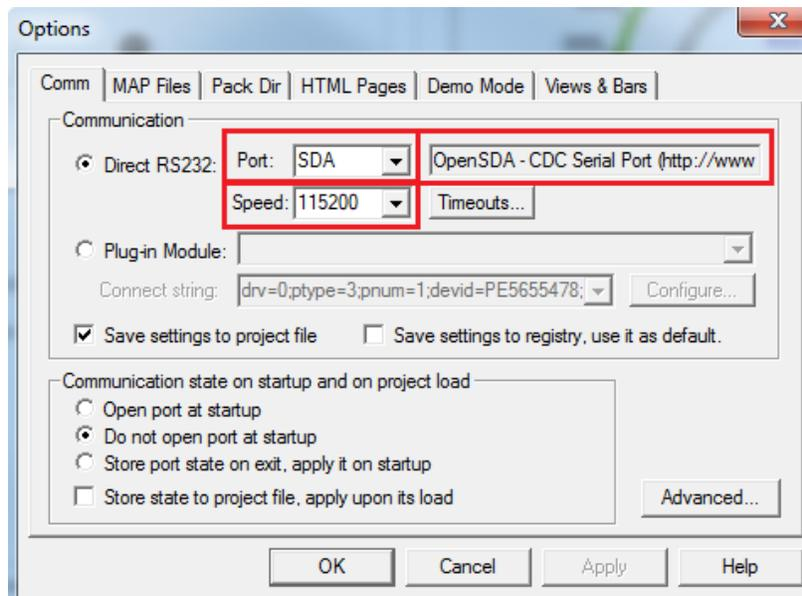
**Figure 23. FreeMASTER communication setup window**
