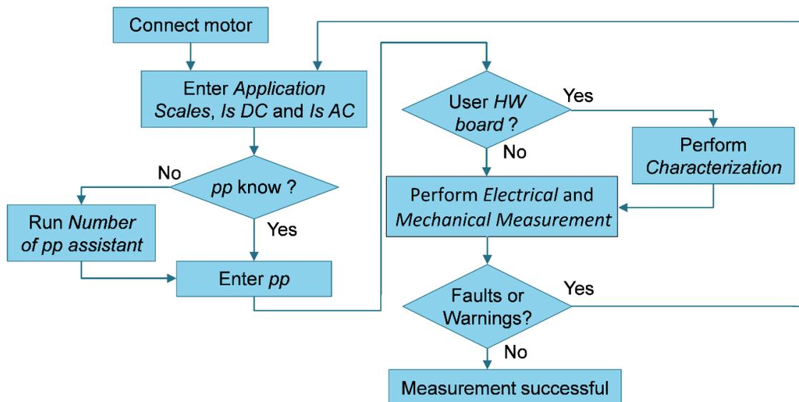
Figure 36. Measurement process diagram
