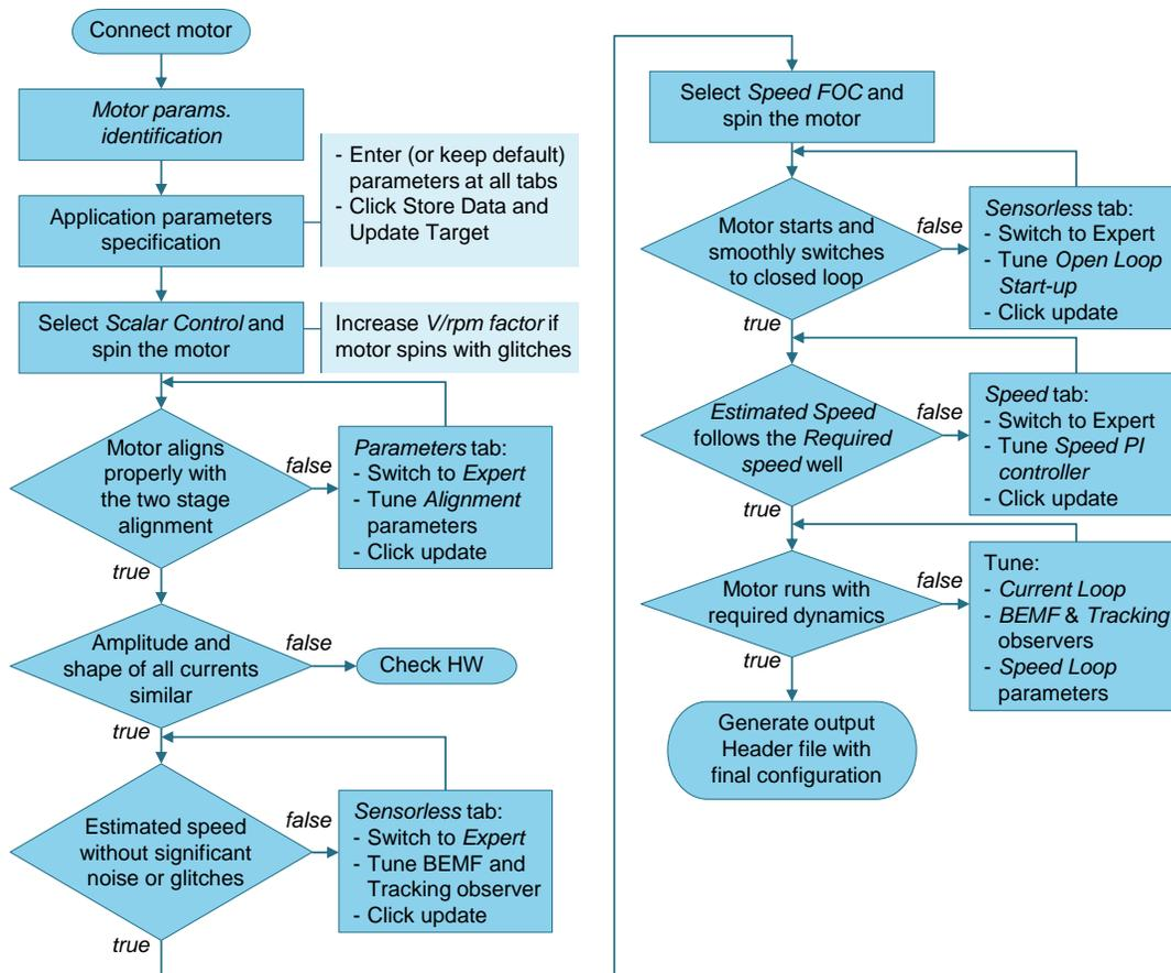
Figure 31. Running a new PMSM
