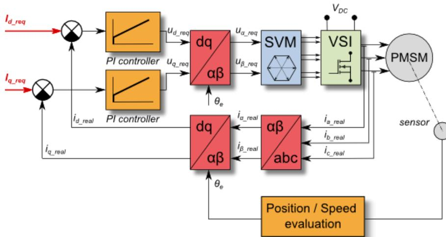
Figure 28. Current (torque) control mode
