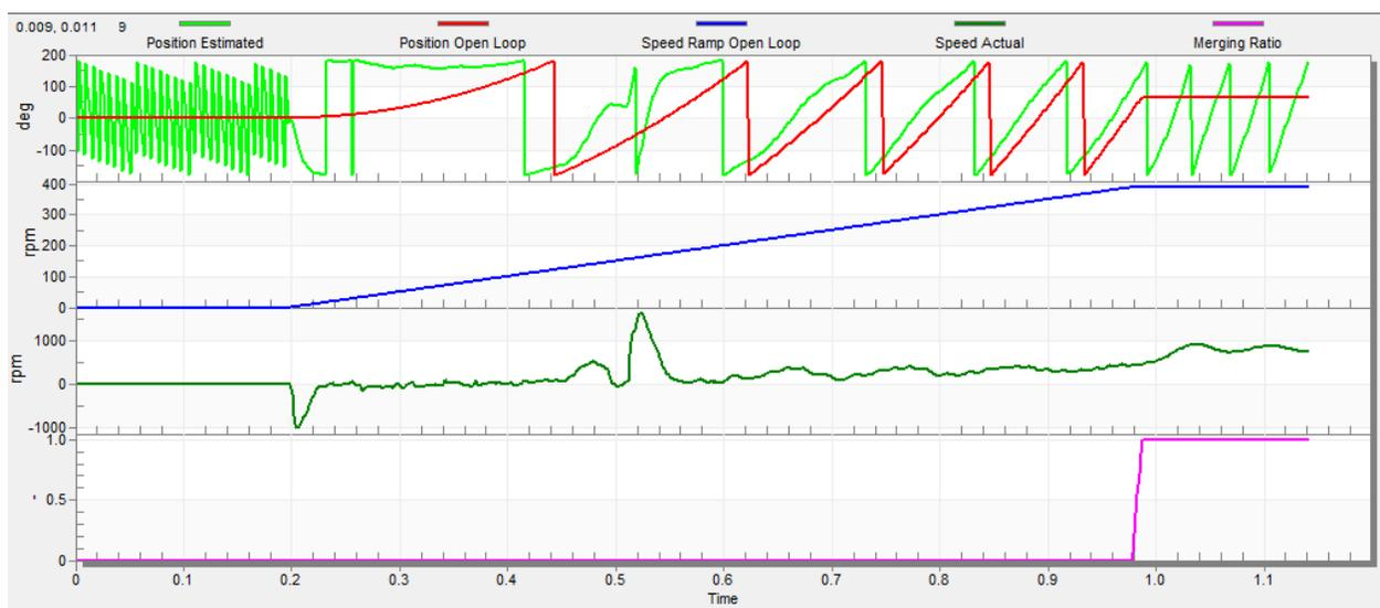
Figure 47. Motor startup
