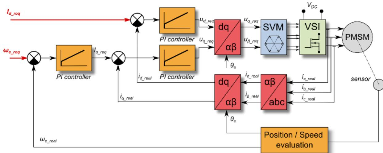
Figure 29. Speed FOC control mode
