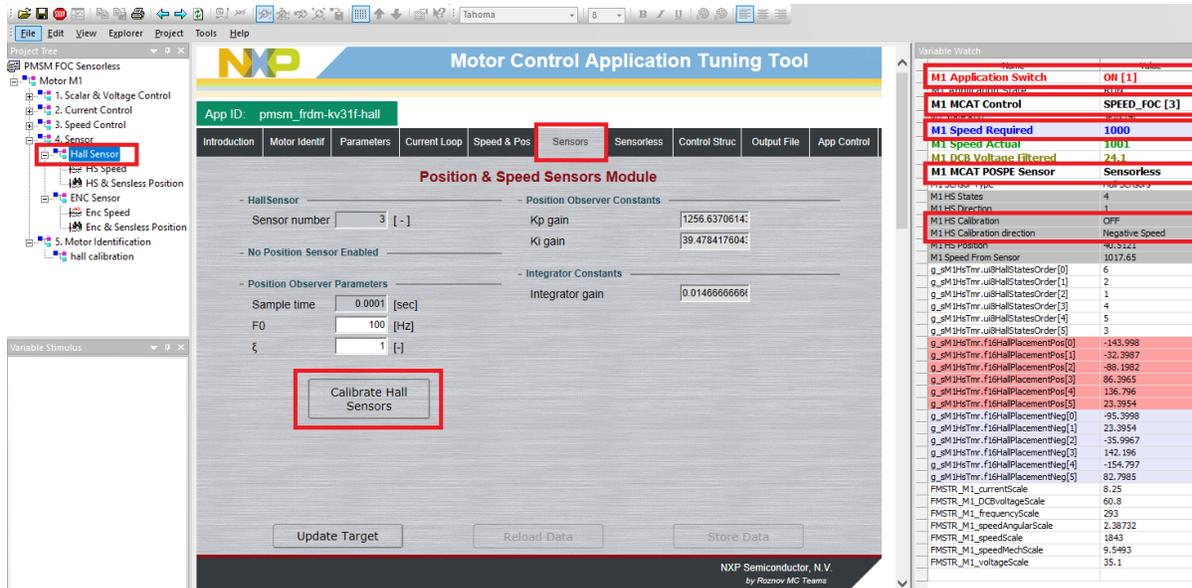
Figure 42. Hall sensors calibration
