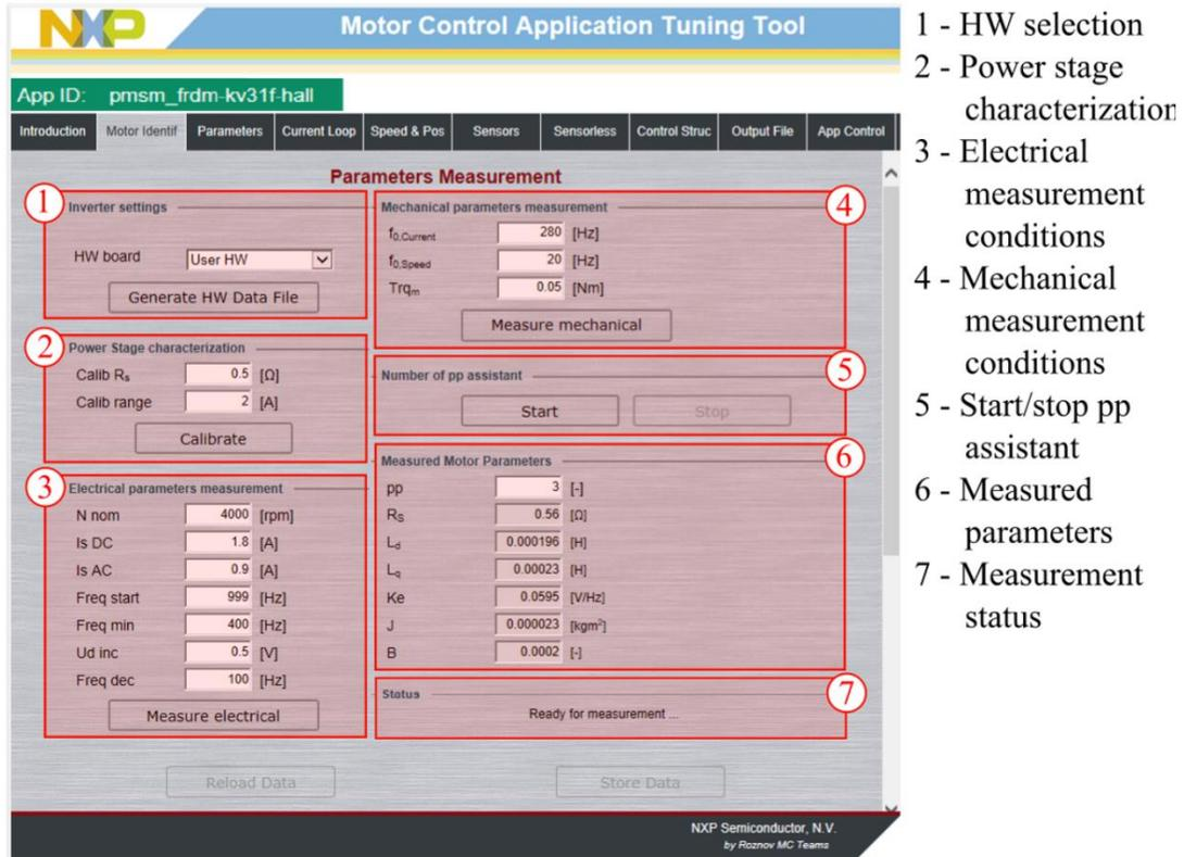
Figure 35. PMSM identification tab
