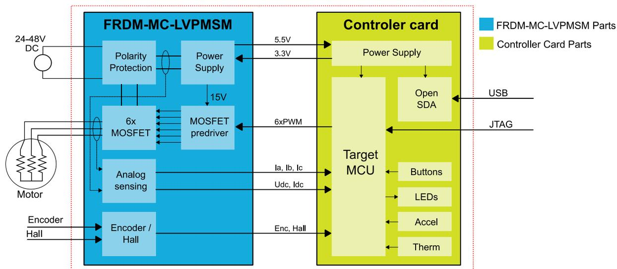
Figure 2. Motor-control development platform block diagram
