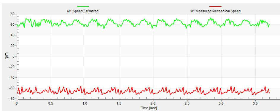
Figure 41. Encoder direction—wrong direction
