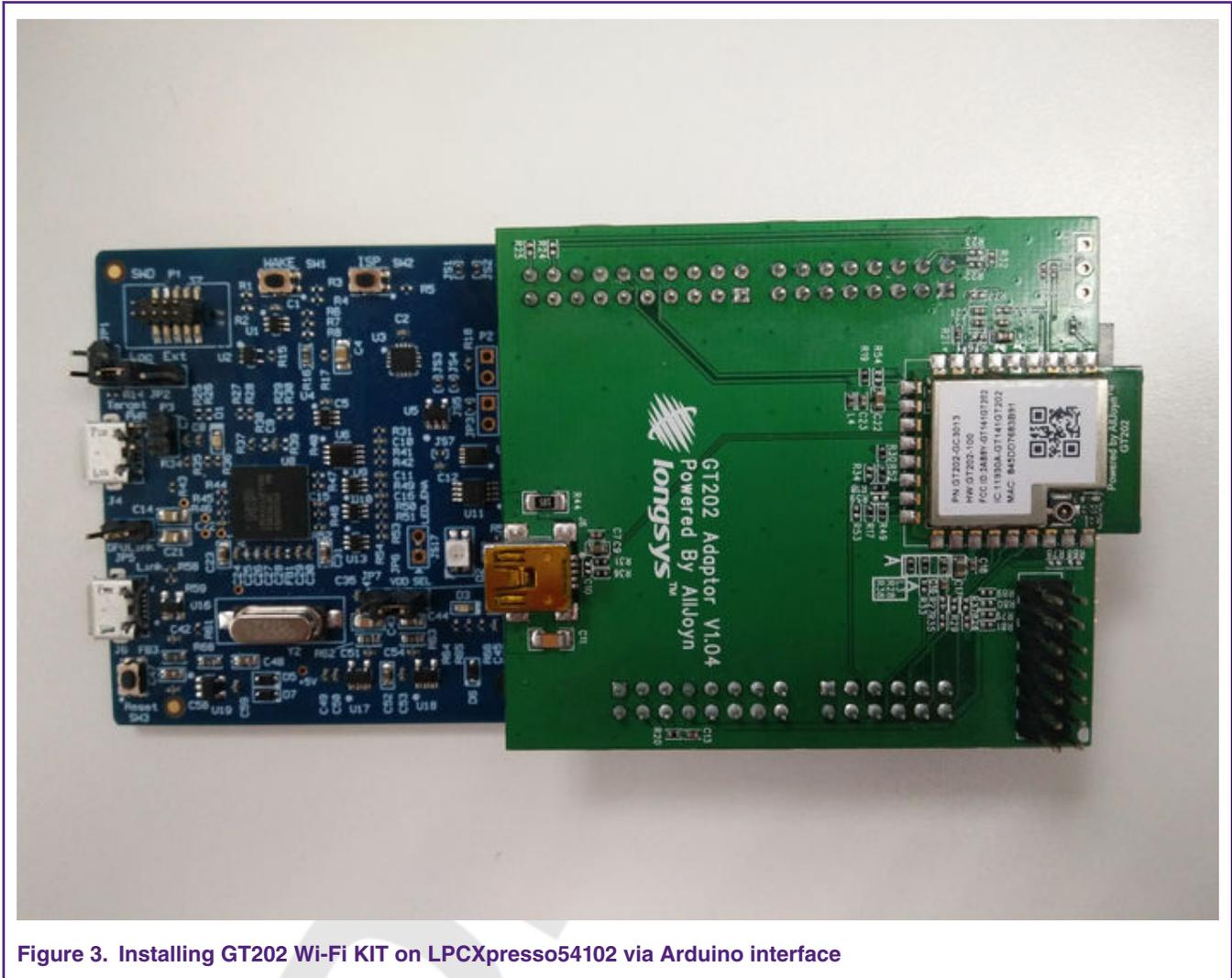
**Figure 3. Installing GT202 Wi-Fi KIT on LPCXpresso54102 via Arduino interface**
