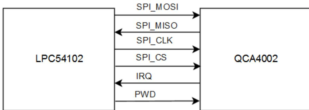
Figure 4. Hardware connection between LPC54102 and QCA4002
