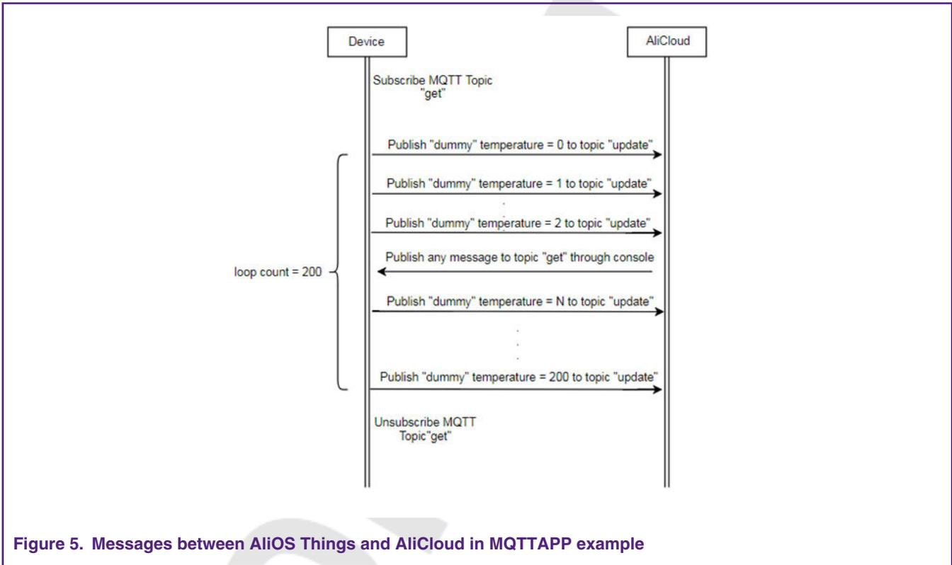
Figure 5. Messages between AliOS Things and AliCloud in MQTTAPP example
