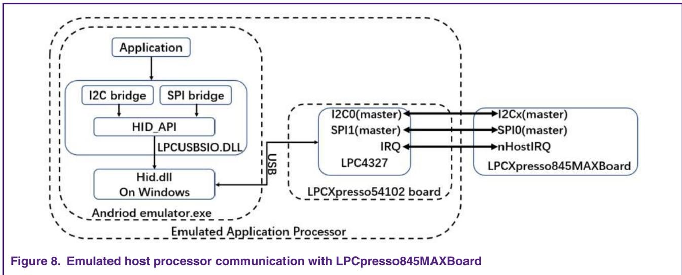
**Figure 8. Emulated host processor communication with LPCpresso845MAXBoard**
