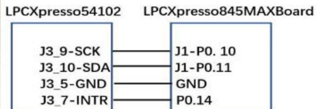
Figure 6. Connection between LPCXpresso 54102 board and LPCXpresso 845 board
