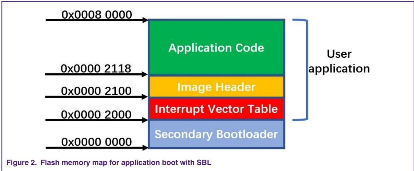
Figure 2. Flash memory map for application boot with SBL
