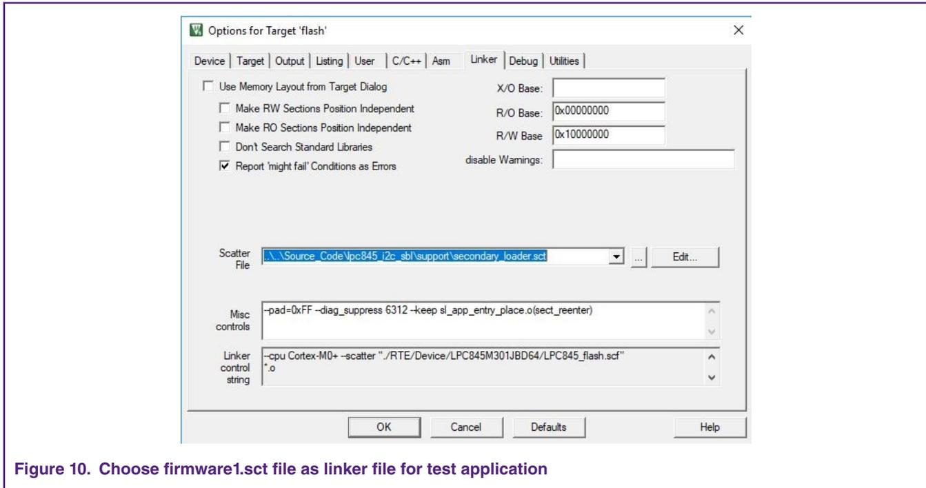
Figure 10. Choose firmware1.sct file as linker file for test application
