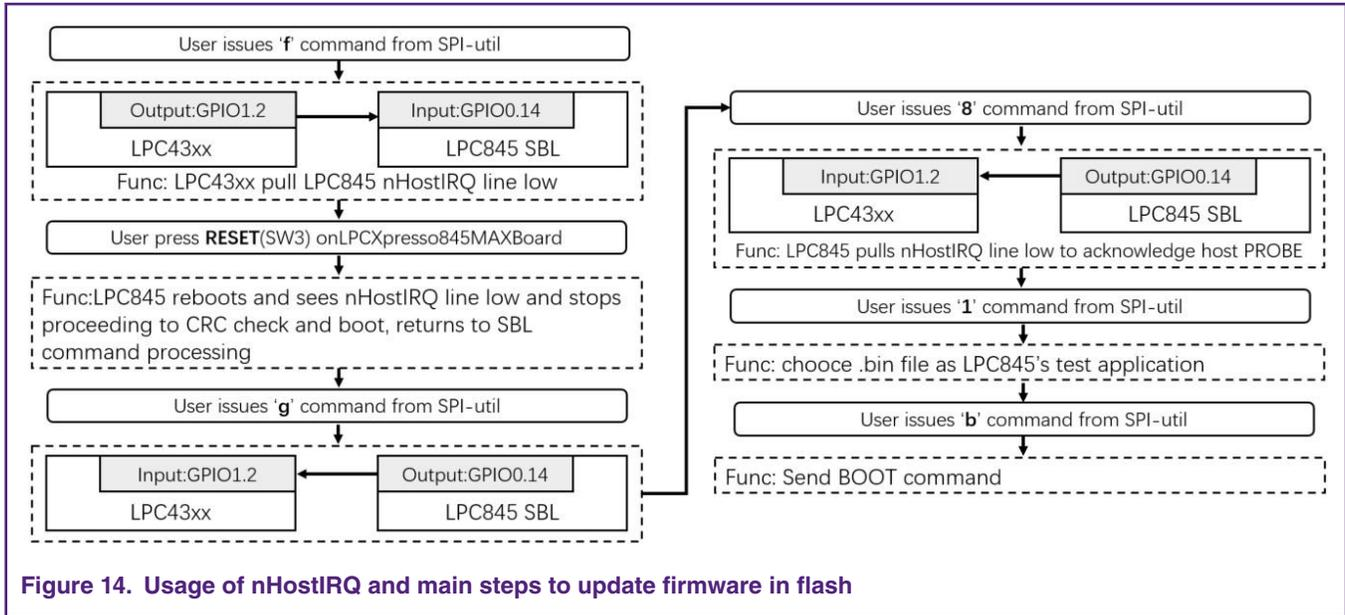
**Figure 14. Usage of nHostIRQ and main steps to update firmware in flash**
