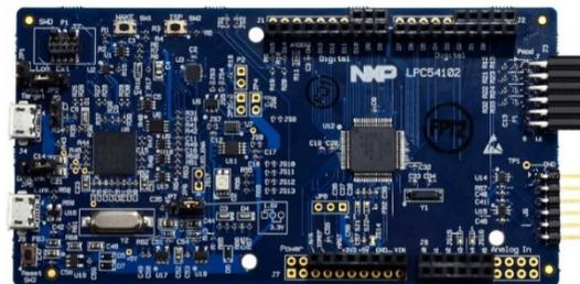
Figure 5. LPCXpresso 54102 board as USB-to-I2C tool
