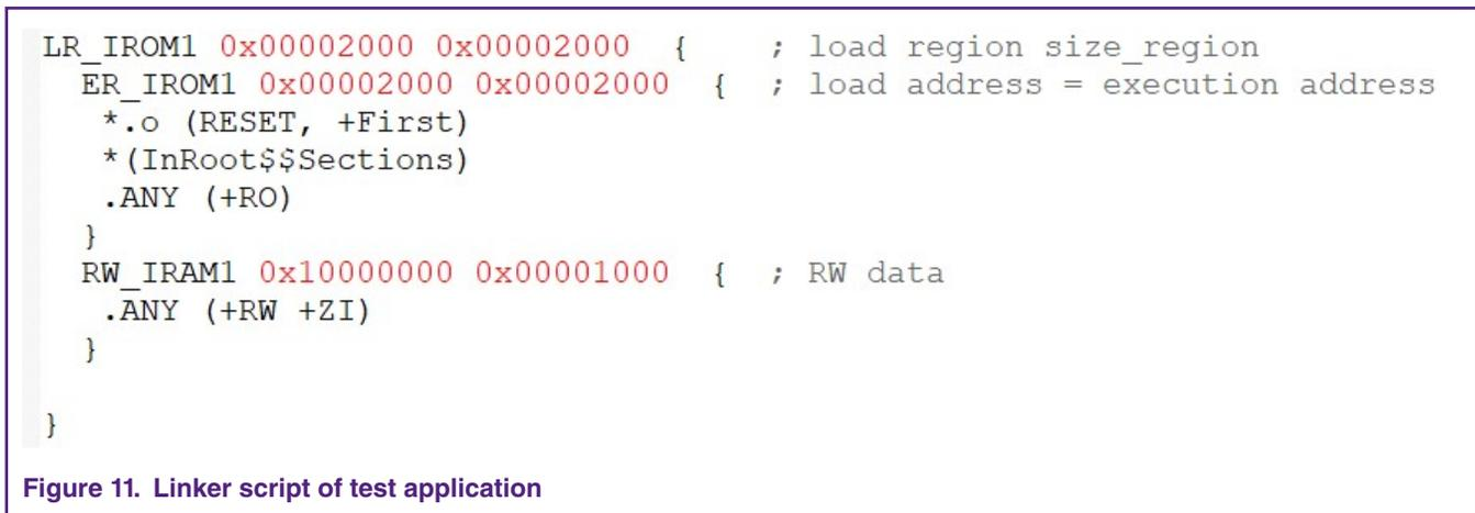
Figure 11. Linker script of test application
