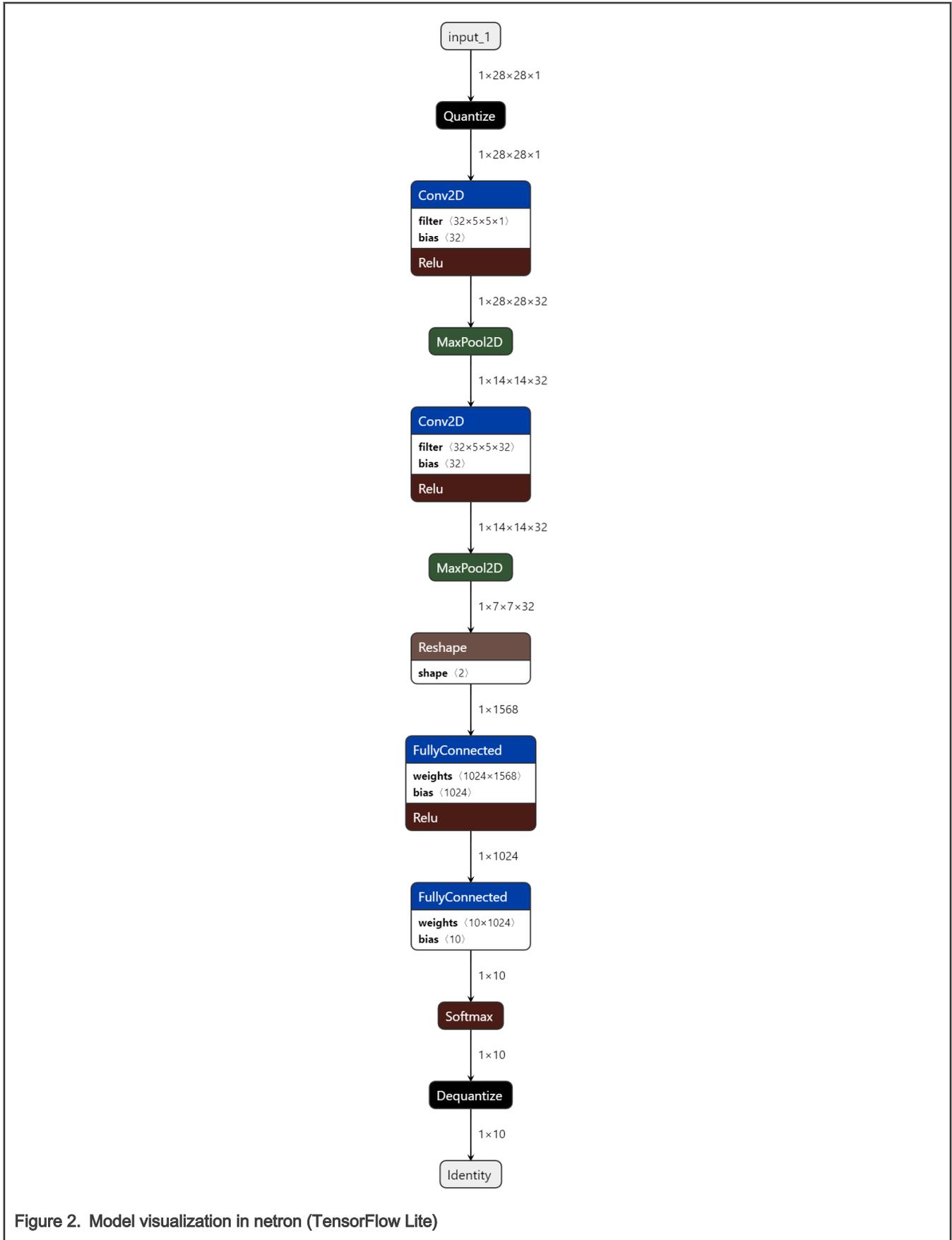
Figure 2. Model visualization in netron (TensorFlow Lite)
