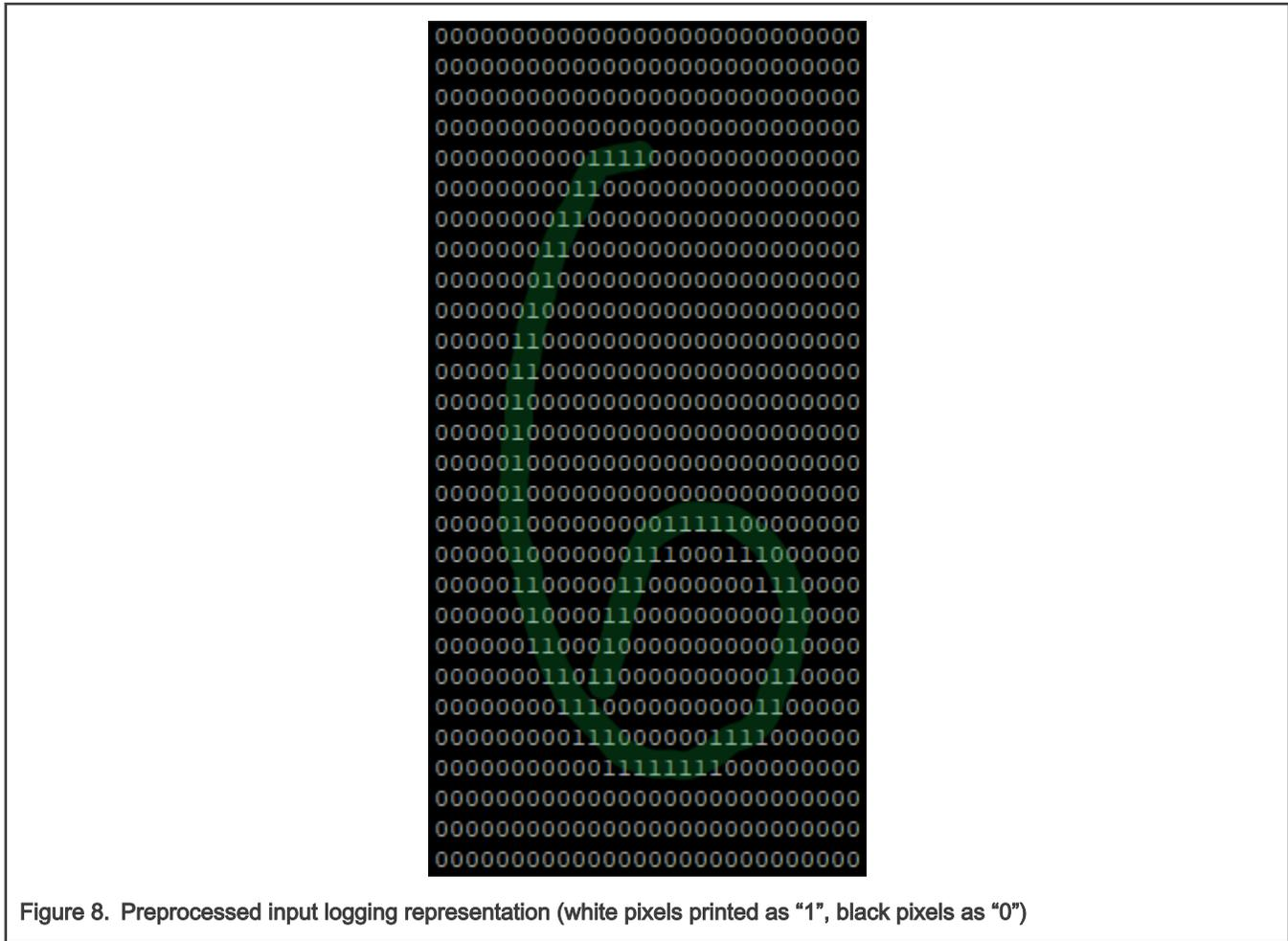
Figure 8. Preprocessed input logging representation (white pixels printed as “1”, black pixels as “0”)
