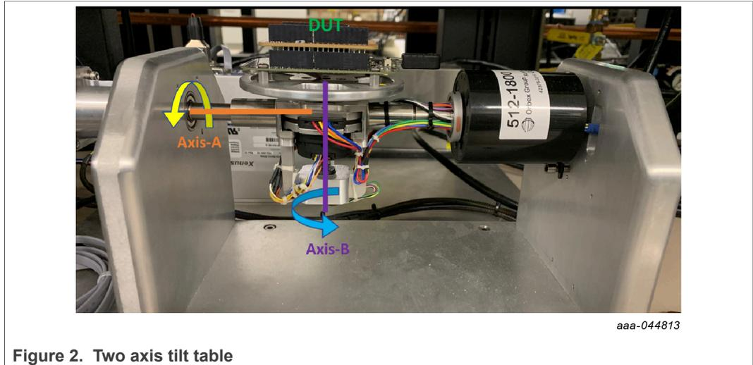
Figure 2. Two axis tilt table
