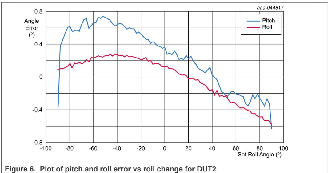
When using a simple sensitivity and offset calibration procedure, the angle accuracy measured on the two FXLS8967 accelerometer samples, is typically better than 1° as observed on the plots.
