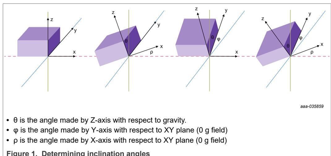
Using basic trigonometry, the following equations are derived:
