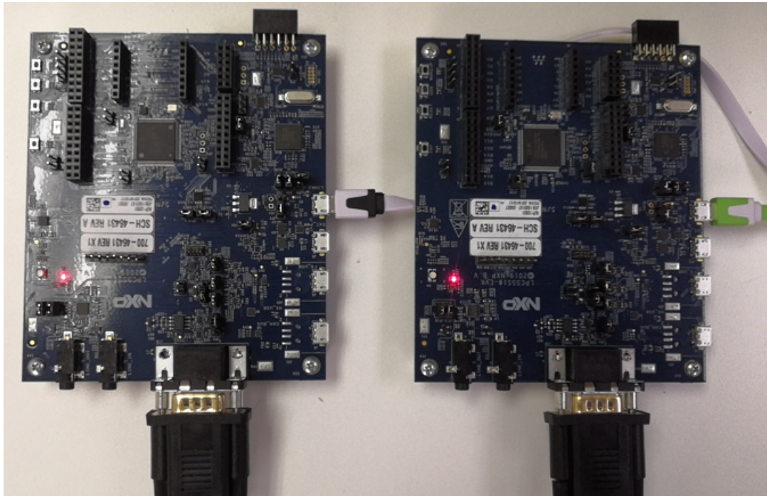
Figure 2. Boards setup and CAN connection
