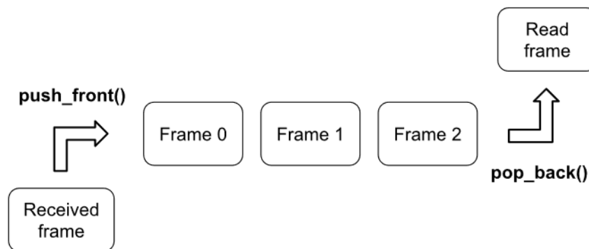
Figure 9. FIFO mechanism for frame reception implemented with a C++ STL deque
