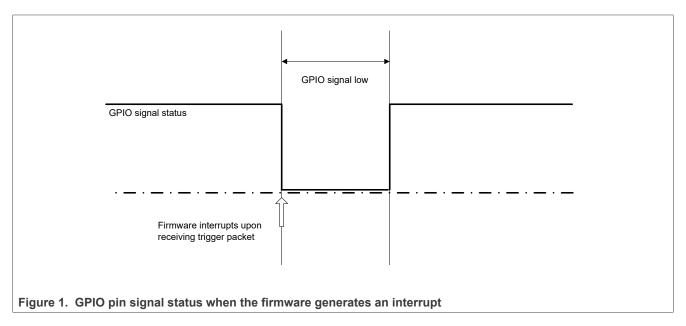
For wireless products with SDIO-SDIO host configuration, the GPIO pin is pulled active low for the GPIO\_GAP time duration. For example:  $gpio_gap=n$ , bits[16:8] =  $GPIO_gap=n$  and bits[8:0] =  $GPIO_gap=n$
