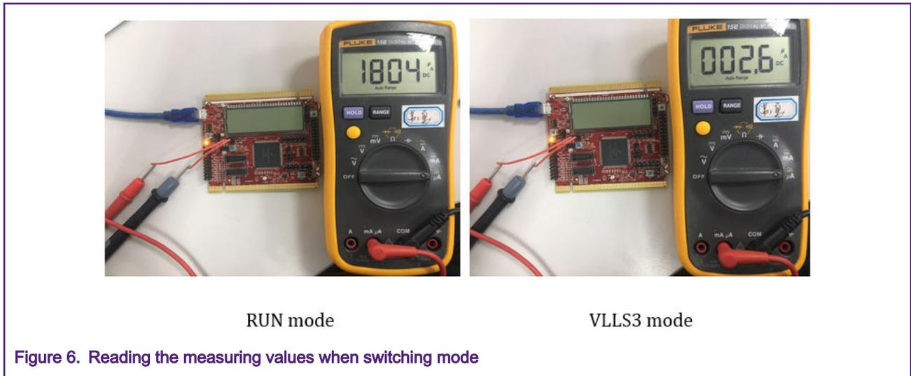
Figure 6. Reading the measuring values when switching mode
