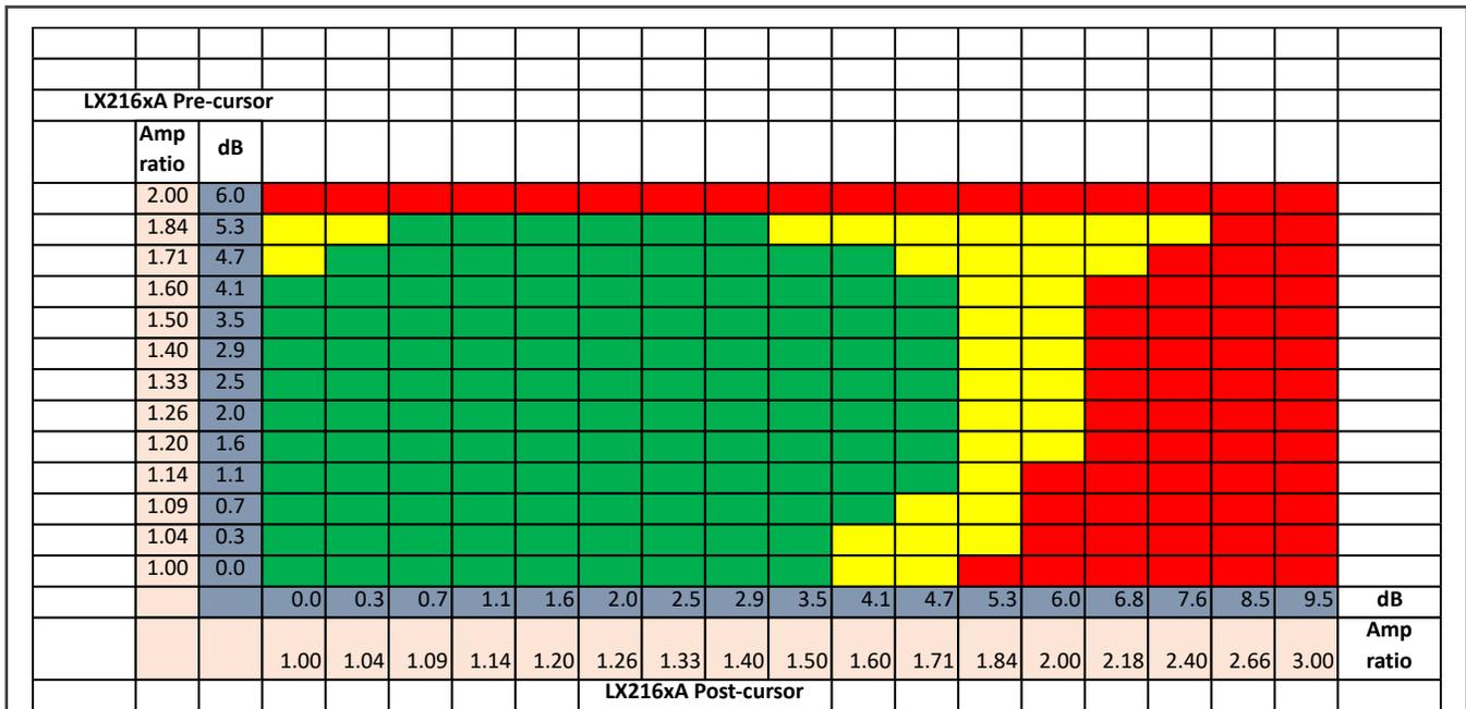
Figure 9. Example of a connected device response to LX216xA transmit equalization tuning
