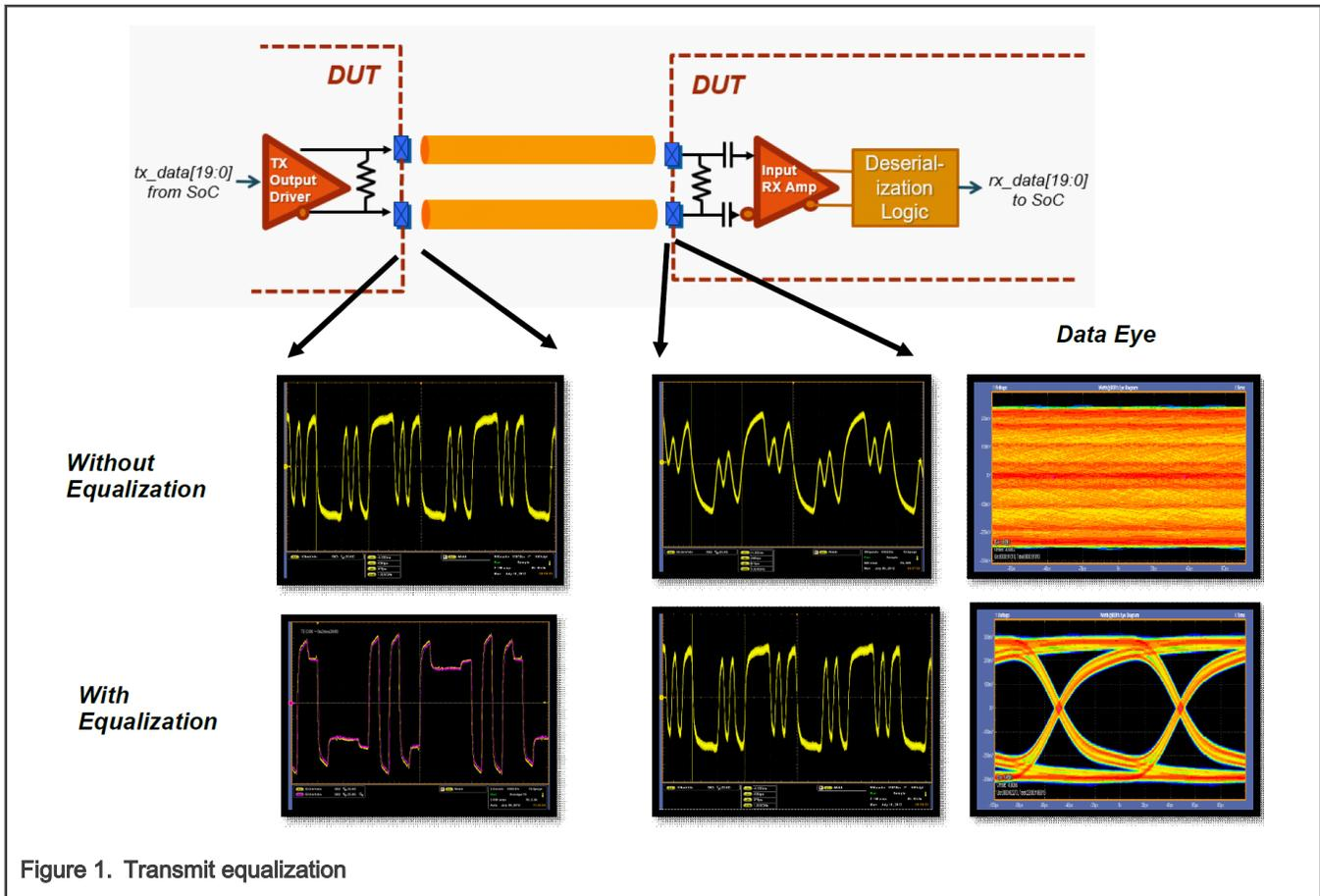
Figure 1. Transmit equalization
