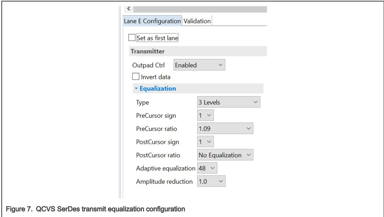
Figure 7. QCVS SerDes transmit equalization configuration
