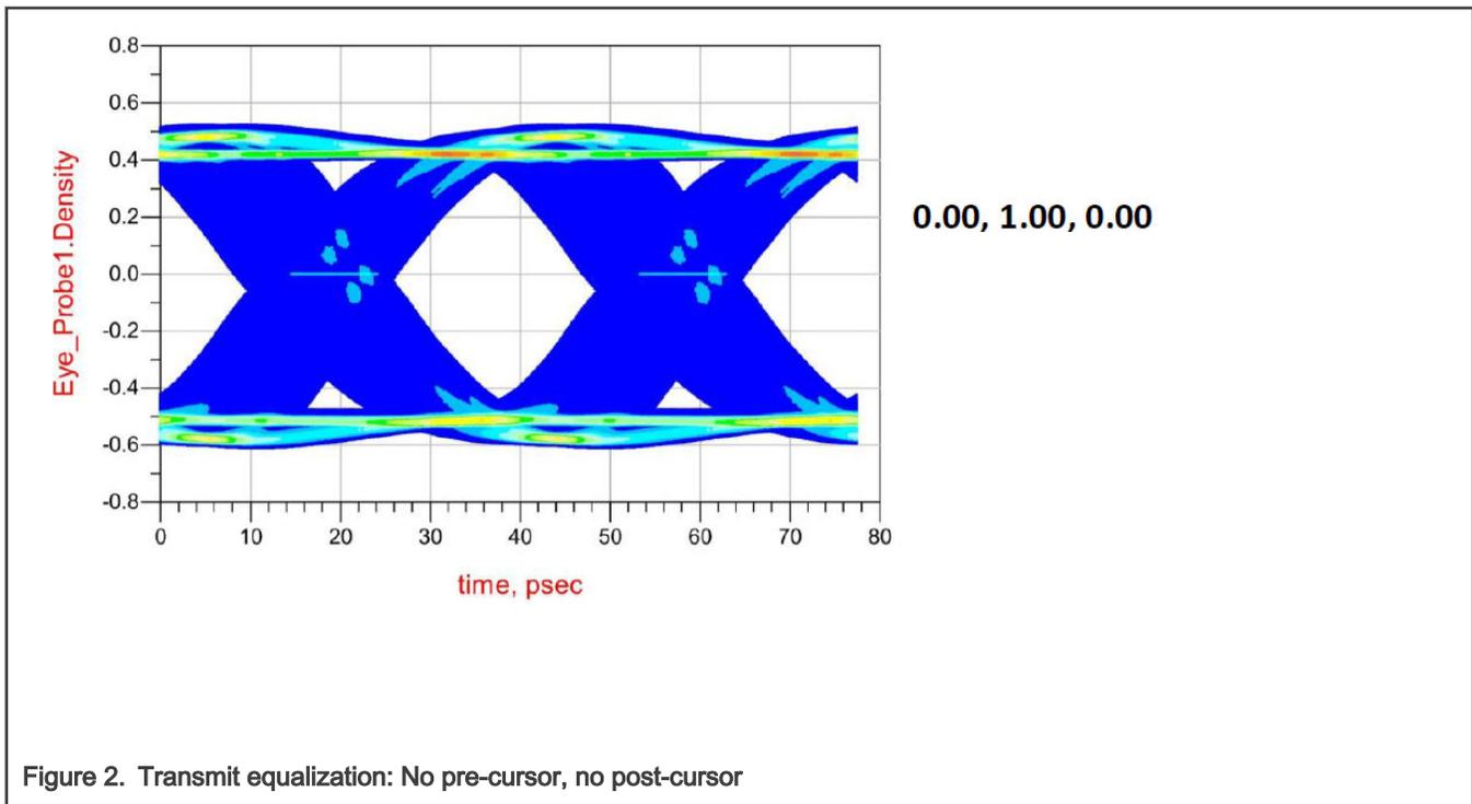
Figure 2. Transmit equalization: No pre-cursor, no post-cursor
