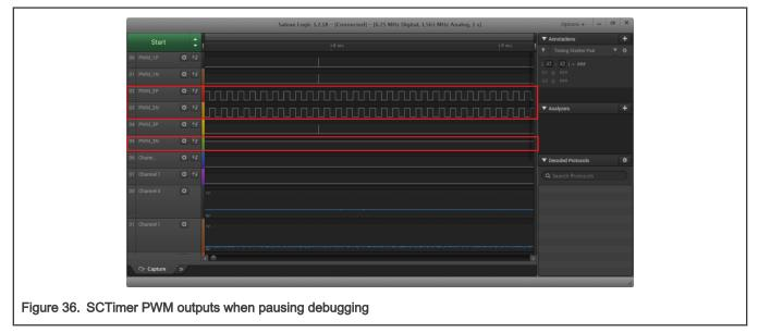
As shown in Figure 3 and Figure 36, PWM\_2P and PWM\_2N which consist of one complementary PWM pair are applied on Q2T and Q2B MOS transistors. Meanwhile, PWM\_3N which is a constant high level is applied on Q3B. Refer to Table 2 and this means that the current flows into the motor B-phase winding and flows out of the C-phase winding. If the high PWM duty cycle causes the phase current to be more than 2A, the motor may heat up in a short time.
