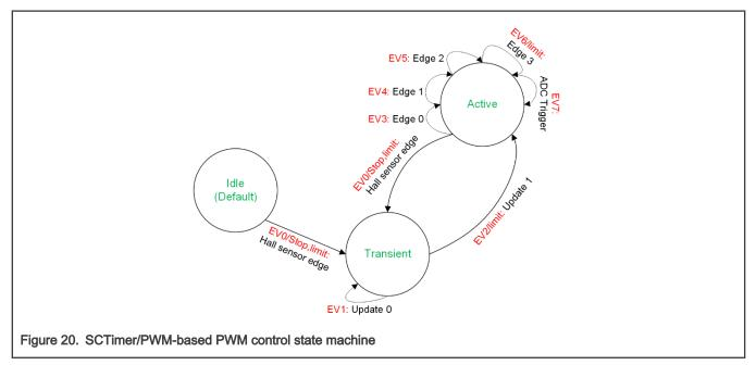
As shown in Figure 20, this state machine consists of three states: Idle, Transient and Active, and eight events, EV0 to EV7.
