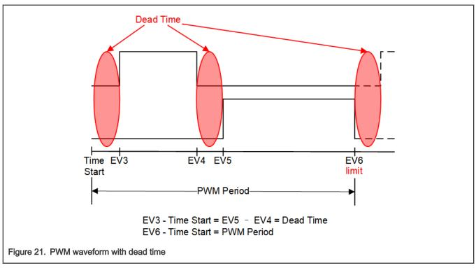
This document adopts edge-aligned mode to generate PWM with dead time and the waveform details are as shown in Figure 21.
