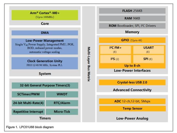
As the peripheral only available in NXP MCUs, the state configurable timer (SCTimer/PWM) is available on all LPC51U68 devices. It can work like traditional timer as a timer/counter. However, unlike traditional timer, a state machine is introduced to SCTimer/PWM. This is the most outstanding feature of SCTimer/PWM and it greatly enhances the configuration and control flexibility of LPC devices. Thanks to this feature, SCTimer/PWM is allowed to support multi-channel PWM with dead-time.
