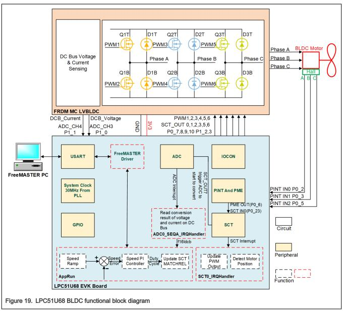
As shown in Figure 19, the overall control process of LPC51U68 BLDC application is mainly completed by the following three parts:
