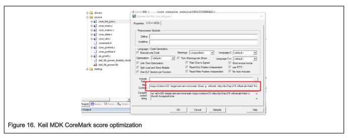
When benchmarking the power consumption of the MCU, the optimization setting must be set to Level 0 (-O0) and **Optimized for time** must be unchecked.
