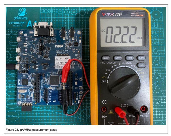
Users can measurement the current through JP22 with a multimeter.
