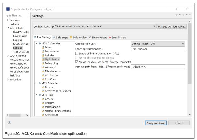
When benchmarking the power consumption of the MCU, set the optimization level to None(-O0).
