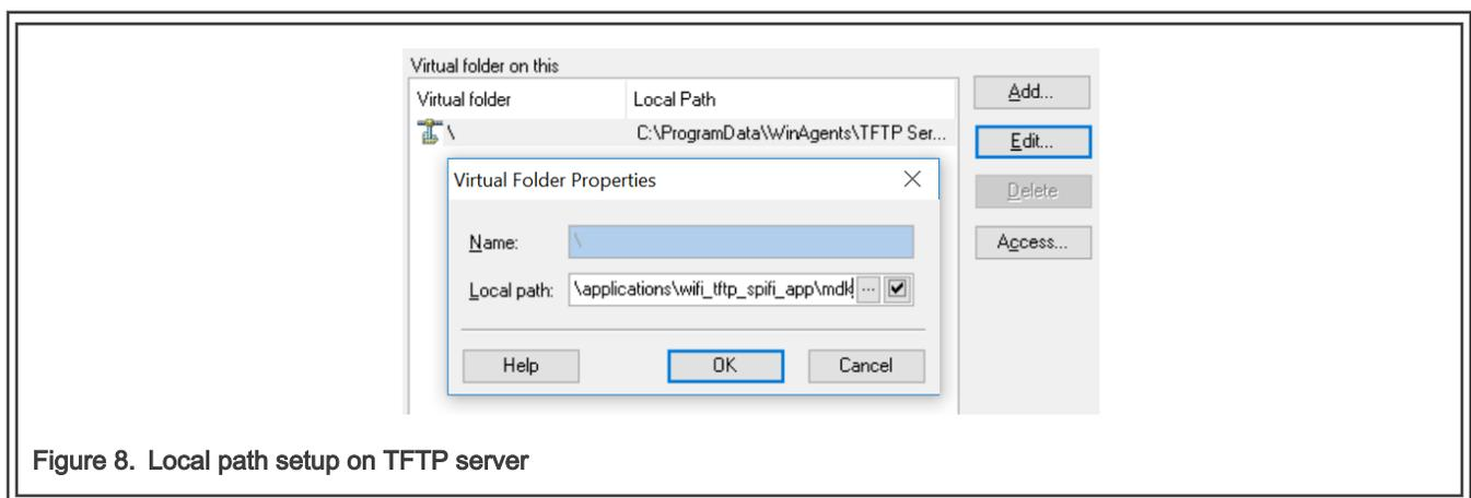
Figure 8. Local path setup on TFTP server
