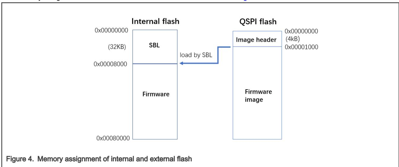
Figure 4. Memory assignment of internal and external flash
