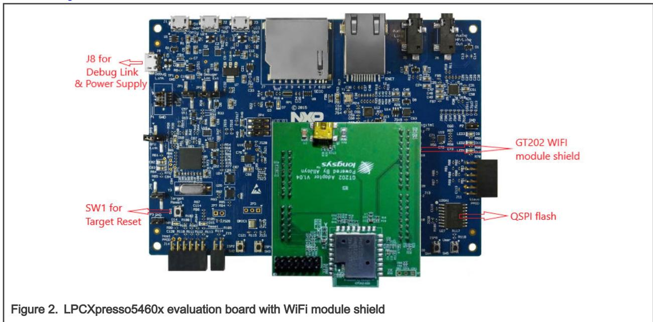
Figure 2. LPCXpresso5460x evaluation board with WiFi module shield
