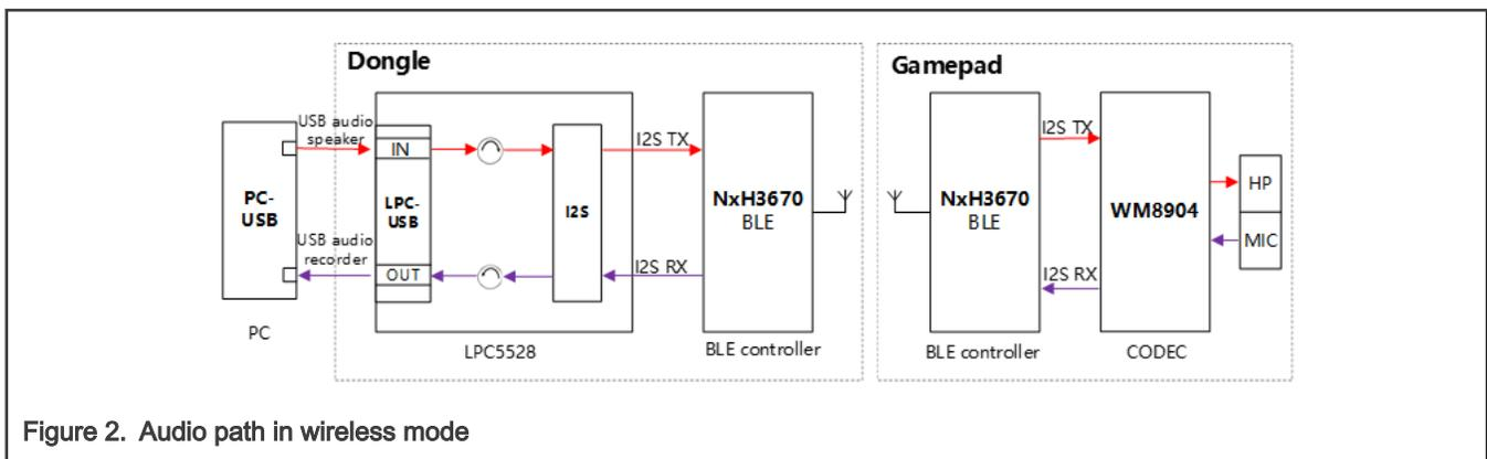
Figure 2. Audio path in wireless mode
