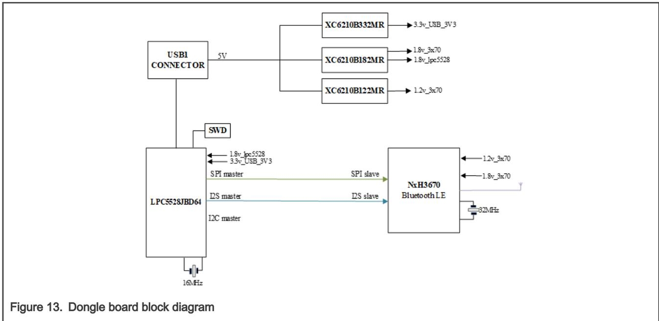
Figure 13. Dongle board block diagram
