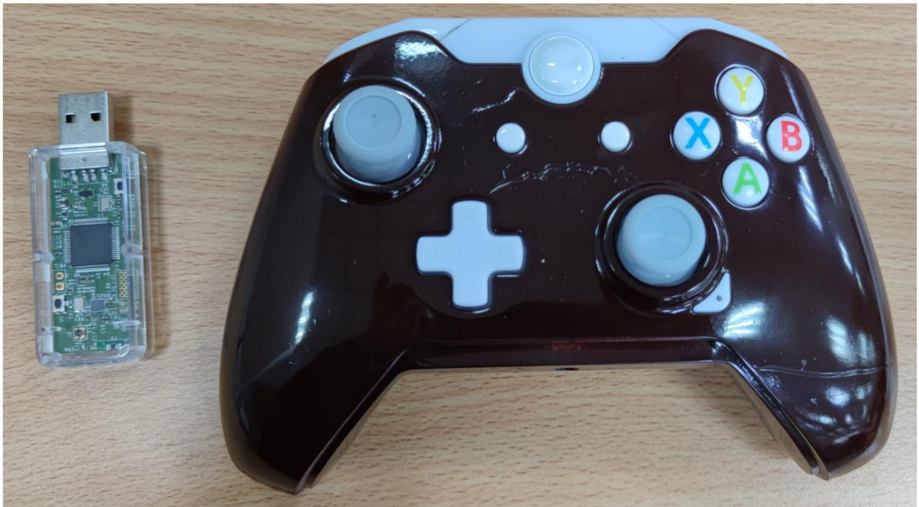
Figure 15. Gamepad board and dongle board after assembly
