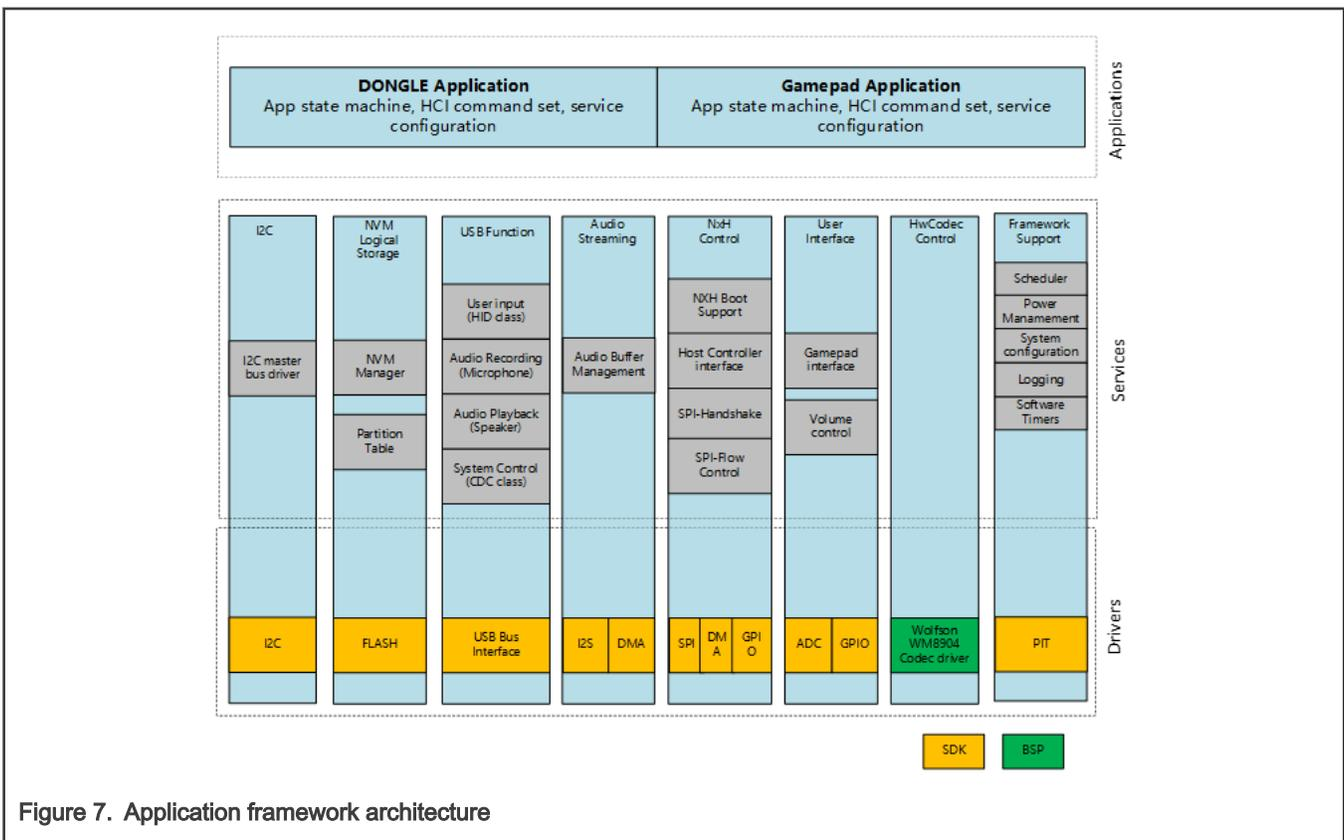
Figure 7. Application framework architecture
