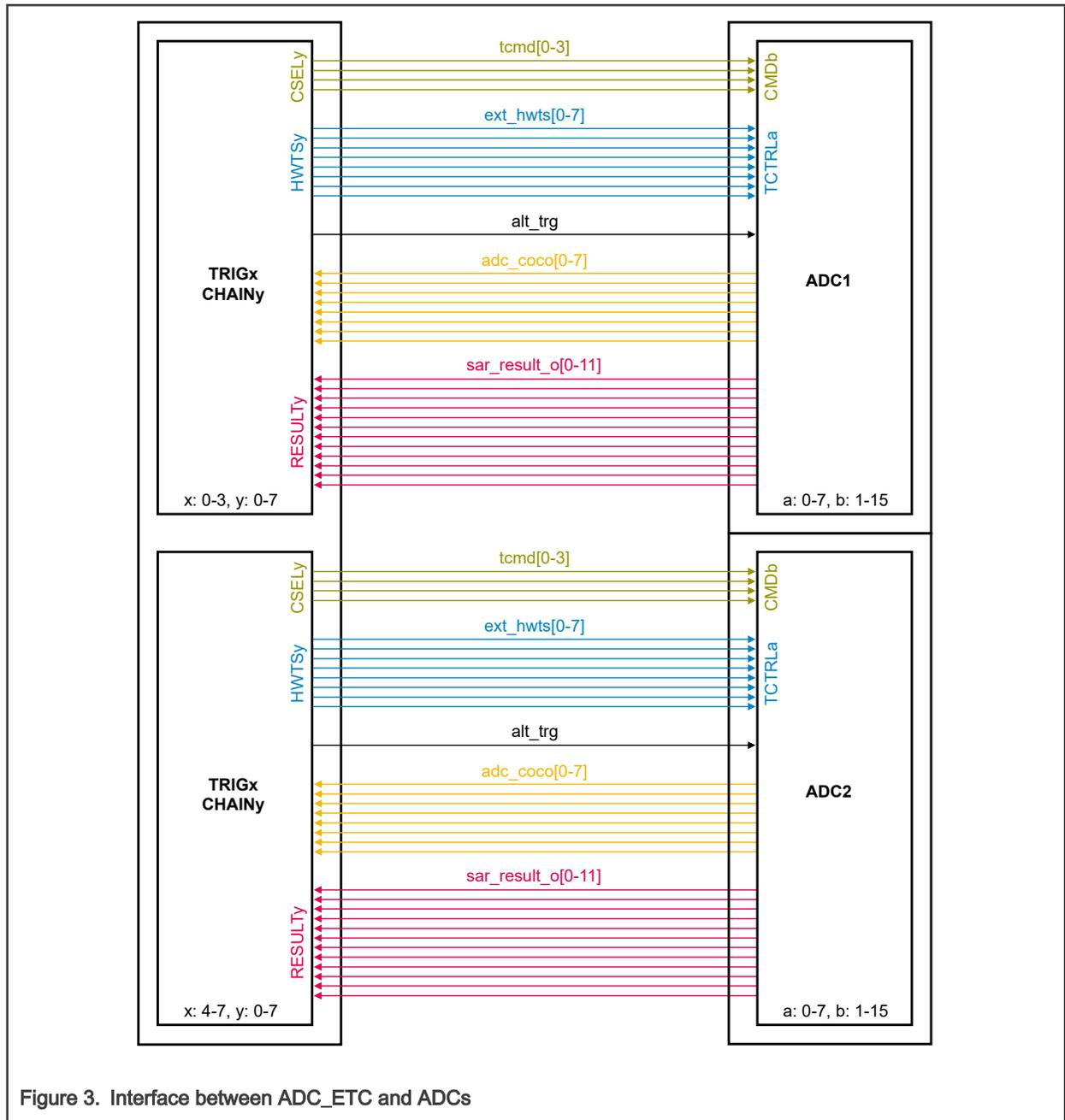
Figure 3. Interface between ADC\_ETC and ADCs
