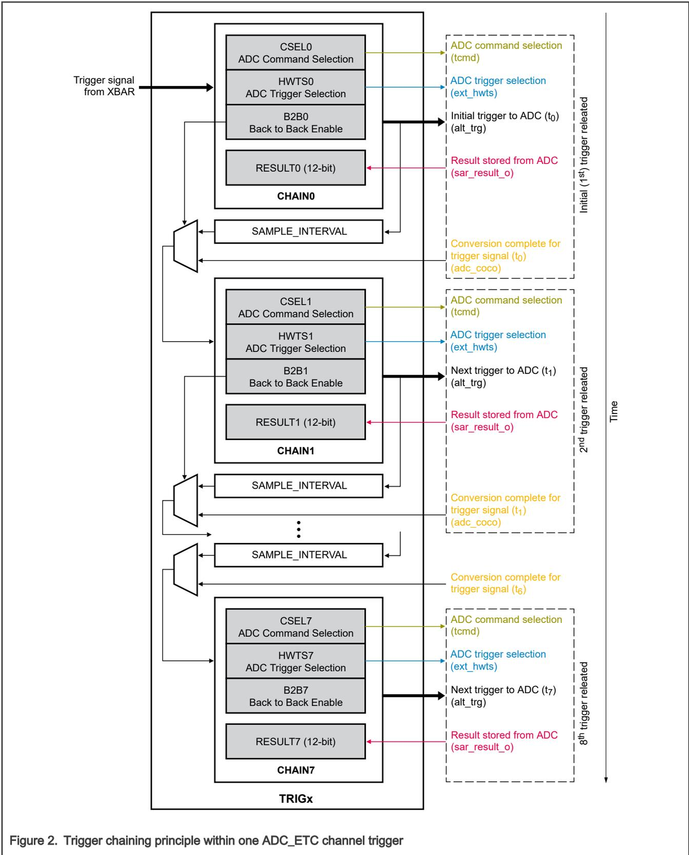
Figure 2. Trigger chaining principle within one ADC\_ETC channel trigger
