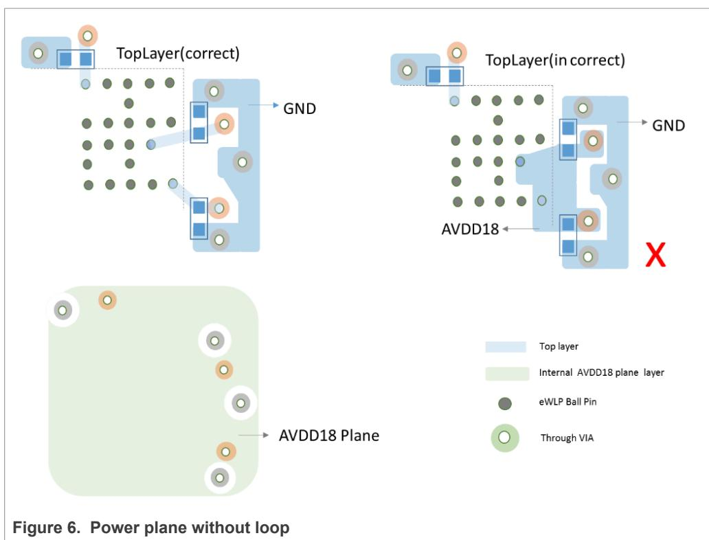
Figure 6. Power plane without loop
